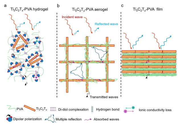
Fig. 6 Schematic illustrations of the EMI shielding mechanism in (a)  $T_{i_3}C_2T_x$ -PVA hydrogels, (b)  $T_{i_3}C_2T_x$ -PVA aerogels, and (c)  $T_{i_3}C_2T_x$ -PVA compact films. The diagrams highlight the key factors contributing to EMI shielding performance reflection, absorption, and internal multiple reflections and their respective roles in attenuating electromagnetic waves.
