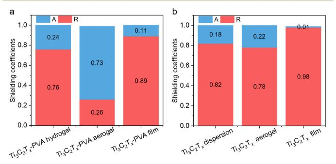
Fig. 5 Absorption coefficient (A) and reflection coefficient (R) of the (a) Ti<sub>3</sub>C<sub>2</sub>T<sub>x</sub>-PVA-based hydrogel, aerogel, and film and (b) Ti<sub>3</sub>C<sub>2</sub>T<sub>x</sub>-based dispersion, aerogel, and film at a fixed  $Ti_3C_2T_x$  areal density (20 mg cm<sup>-2</sup>).
