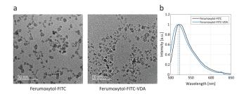
Fig. 1 Electron microscopy and optical fluorescence. (a) TEM micrograph of Ferumoxytol-FITC showing the dispersed iron oxide cores. Scale bars, 50 nm. (b) Optical fluorescence spectra of Ferumoxytol-FITC and Ferumoxytol-FITC-VDA, employing an excitation wavelength of 480 nm, and yielding emission peaks at 521 and 517 nm, respectively.
