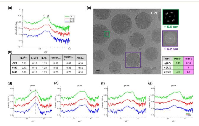
Fig. 7 SAXS diffractograms (a) and peak features (b) of the OPT, Std 2, and Std 1 formulations in 10% Trehalose. (c) Shows Cryo-TEM image, FFT profiles, and *d*-spacing of the multilamellar (purple box) and inverted hexagonal (green box) structures of the OPT formulation. SAXS diffractograms (d–g) of the OPT, Std 2, and Std 1 formulations mixed with citrate-phosphate buffers at different pH values.
