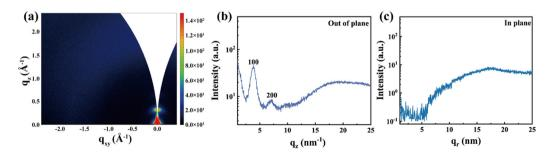
Fig. 4 GIWAXS analysis. (a) 2D GIWAXS pattern. (b) Out of plane  $(q_z)$  and (c) in plane  $(q_t)$  orientation integrations of PDPP-TEG-2Tz, as derived from 2D GIWAXS.
