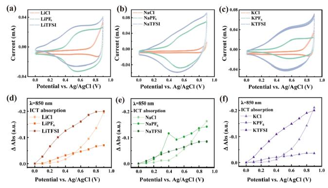
Fig. 5 Cyclic voltammetry (CV) and electrochemical spectroscopy in aqueous electrolyte. (a-c) 10 CV cycles at a scan rate of 100 mV s<sup>-1</sup>, starting from 0 to 0.9 V. (d-f) The evolution of the relative absorption at 850 nm (ICT) as the potential increases.
