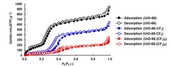
Fig. 3 Water vapor adsorption/desorption isotherms of UiO-66 (black), UiO-66-CF<sub>3</sub> (blue), and UiO-66-(CF<sub>3</sub>)<sub>2</sub> (red) at 298 K. Their crystallinity was maintained after water vapor adsorption (Fig. S5†).
