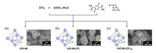
Fig. 1 Preparation and scanning electron microscopy (SEM) images (scale bar: 100 nm) of (a) UiO-66, (b) UiO-66-CF<sub>3</sub>, and (c) UiO-66-(CF<sub>3</sub>)<sub>2</sub>.
