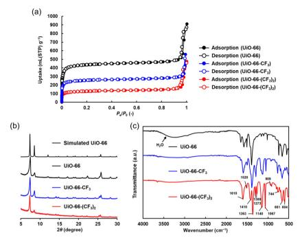
Fig. 2 (a)  $N_2$  adsorption/desorption isotherms of UiO-66 (black), UiO-66-CF<sub>3</sub> (blue), and UiO-66-(CF<sub>3</sub>)<sub>2</sub> (red) at 77 K. Their crystallinity was maintained after  $N_2$  adsorption (Fig. S5†). (b) PXRD patterns of simulated UiO-66 (upper black), UiO-66 (lower black), UiO-66-CF<sub>3</sub> (blue), and UiO-66-(CF<sub>3</sub>)<sub>2</sub> (red). (c) FT-IR spectra of UiO-66 (black), UiO-66-CF<sub>3</sub> (blue), and UiO-66-(CF<sub>3</sub>)<sub>2</sub> (red).
