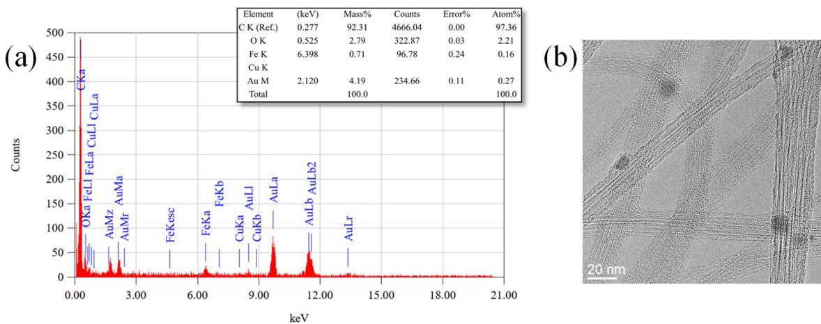
**Fig. 6** EDS analysis of the Cu/Fe 0.5 catalyst nanoparticles. (a) Representative EDS spectrum of the scanned particles and (b) TEM micrograph of the particles in the EDS spectrum.
