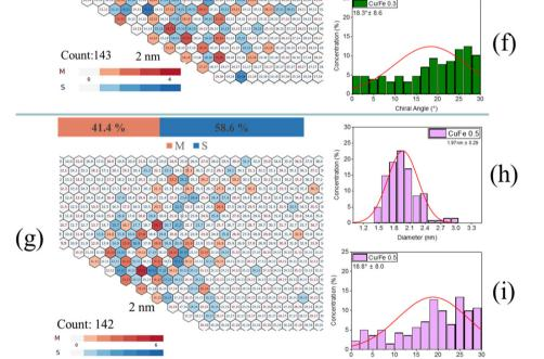
Fig. 7 Chirality maps and the corresponding distributions of diameters and chiral angles for all samples. (a–c) Fe sample, (d–f) Cu/Fe 0.3 sample, and (g–i) Cu/Fe 0.5 sample.
