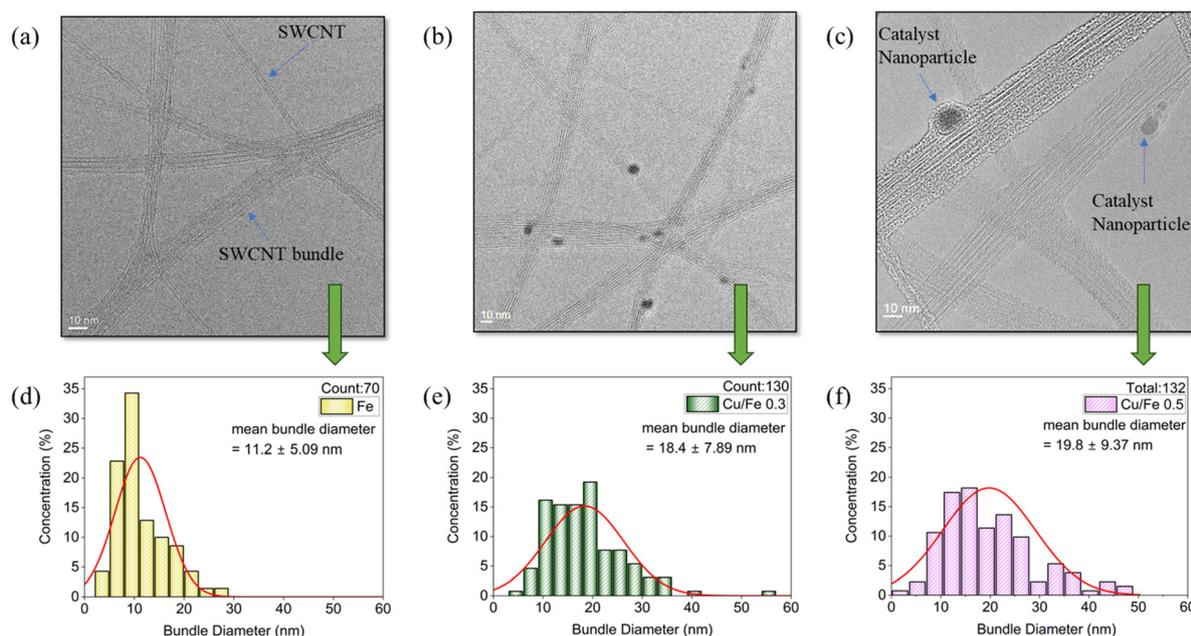
**Fig. 4** TEM morphology characterization of the SWCNTs. (a) TEM micrograph of the Fe sample, (b) TEM micrograph of the Cu/Fe 0.3 sample, (c) TEM micrograph of the Cu/Fe 0.5 sample, (d) bundle diameter distribution of the Fe sample, (e) bundle diameter distribution of the Cu/Fe 0.3 sample, and (f) bundle diameter distribution of the Cu/Fe 0.5 sample.
