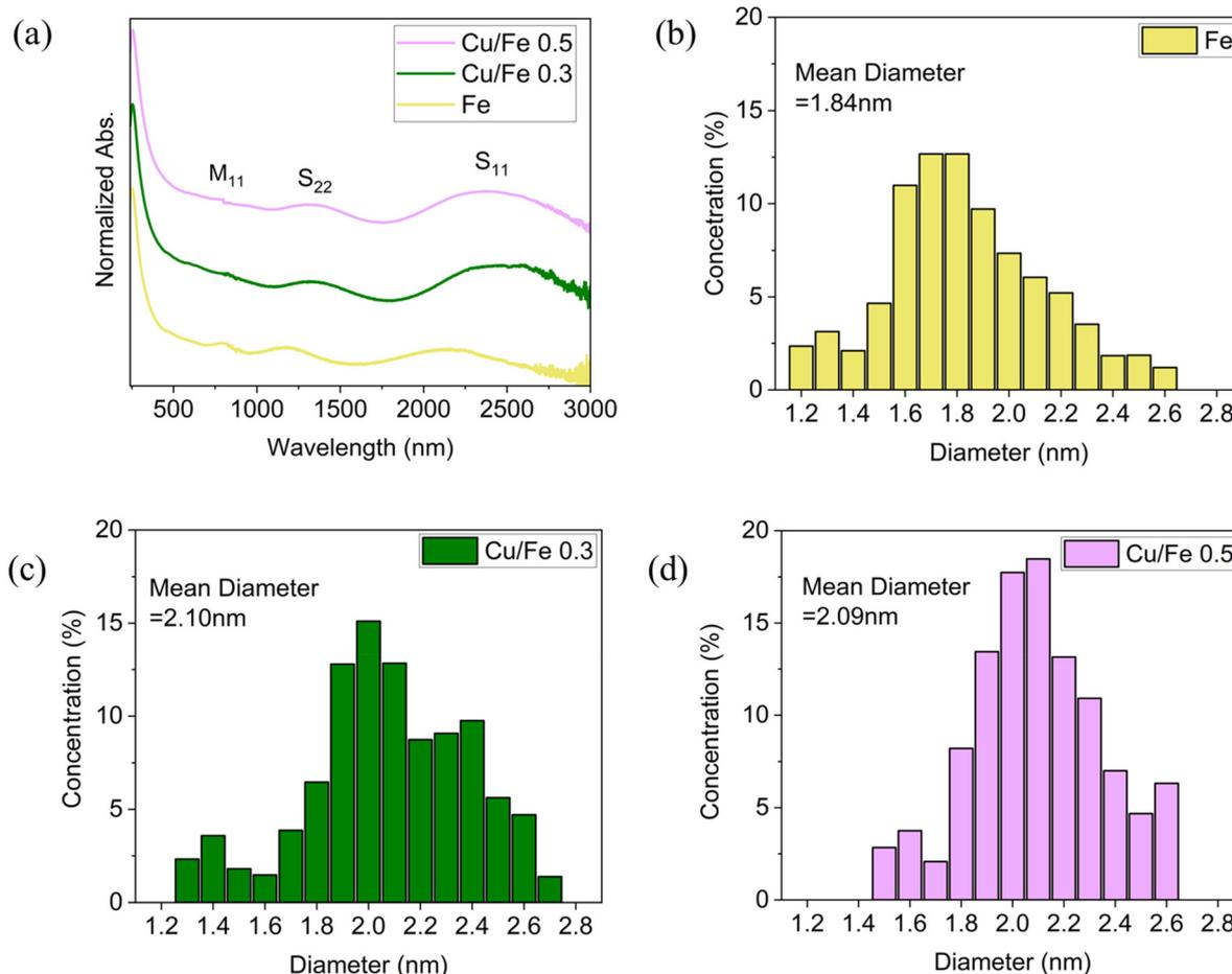
**Fig. 3** UV-vis-NIR assessment of all samples. (a) Light absorption spectra, (b) diameter distribution of the Fe sample, (c) diameter distribution of the Cu/Fe 0.3 sample and (d) diameter distribution of the Cu/Fe 0.5 sample. The diameter distributions in this figure were plotted using a MATLAB code.
