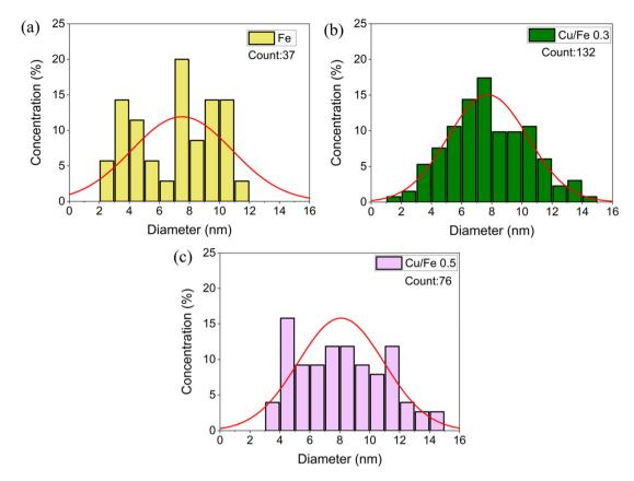
Fig. 5 Nanoparticle diameter distributions of all samples. (a) Fe sample, (b) Cu/Fe 0.3 sample, and (c) Cu/Fe 0.5 sample. The data were analysed from at least 40 individual TEM micrographs for each sample.
