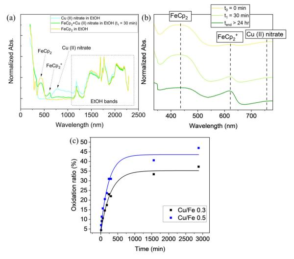
Fig. 2 (a) UV-vis-NIR absorption spectra of all samples, (b) UV-vis-NIR spectra of all samples during the oxidation process, and (c) oxidation ratio (%) of all samples over time.
