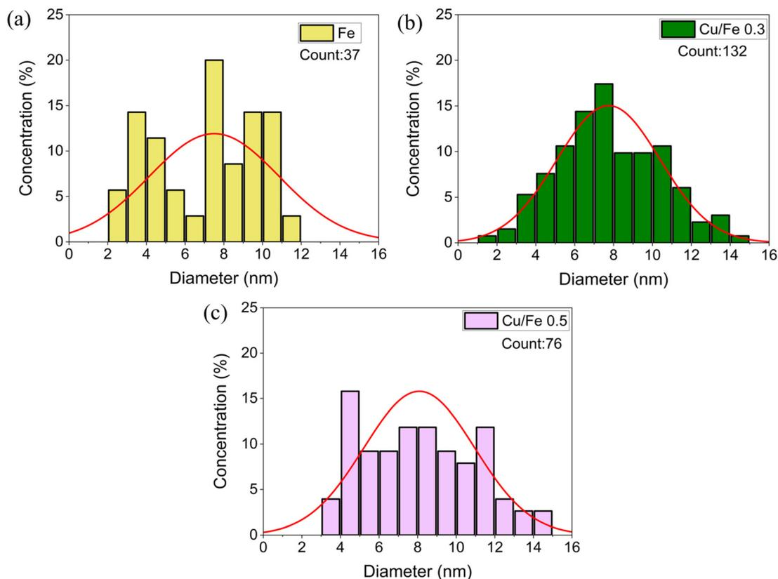
**Fig. 5** Nanoparticle diameter distributions of all samples. (a) Fe sample, (b) Cu/Fe 0.3 sample, and (c) Cu/Fe 0.5 sample. The data were analysed from at least 40 individual TEM micrographs for each sample.
