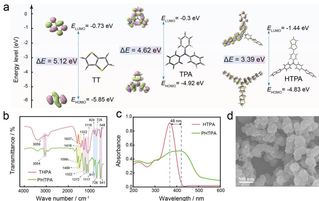
**Fig. 2** Theoretical calculations, structural and morphological characterization of HTPA molecules. (a) Calculation of molecular orbital energies and band gaps of TT, TPA and HTPA using the density functional theory. (b) Comparison of infrared spectra of PHTPA and HTPA. (c) Comparison of infrared spectra of PHTPA and HTPA. (d) SEM images of PHTPA.
