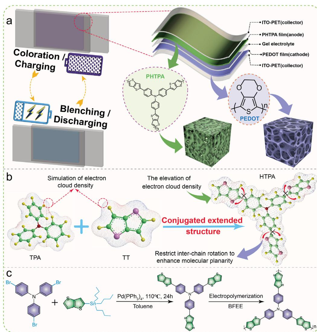
**Fig. 1** (a) Conceptual diagram and application scenarios of PHTPA/PEDOT-based flexible devices. (b) The design strategy of conjugated extended structures. (c) The synthesis pathway of HTPA molecules.
