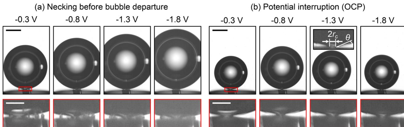
**Fig. 7** Necking process of the bubble base attached to the smoother surface in 1 M  $\text{H}_2\text{SO}_4$ . Images shortly before bubble detachment (a) and shortly after potential interruption, i.e. setting to the open circuit potential (OCP) (b). The potential interruption is performed at a random instant of time. The black scale bars are 200  $\mu\text{m}$  and the white scale bars inside the insets are 50  $\mu\text{m}$ .
