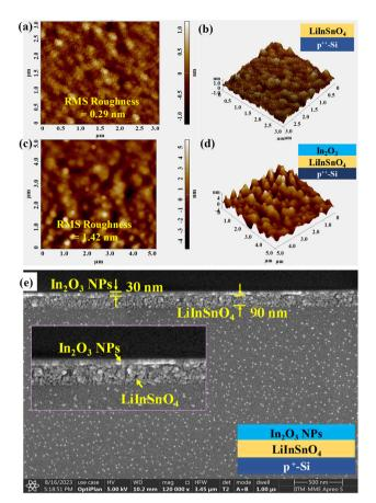
Fig. 3 AFM images: (a) 2D and (b) 3D images of LilnSnO<sub>4</sub> dielectric thin film (p $^+$ -Si/LilnSnO<sub>4</sub>) with  $R_{rms} \sim 0.29$  nm, (c) 2D and (d) 3D images of  $In_2O_3$  NPs thin film (p $^+$ -Si/LilnSnO $_4$ /In $_2O_3$ )  $R_{rms}\sim 1.42$  nm, and (e) crosssectional SEM image of the p<sup>+</sup>-Si/LiInSnO<sub>4</sub>/In<sub>2</sub>O<sub>3</sub> NP film.
