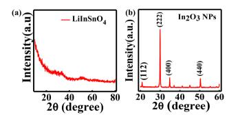
Fig. 1 (a) GIXRD pattern of LilnSnO $_4$  thin film, indicating its amorphous phase and (b) GIXRD pattern of  $In_2O_3$  nanoparticles thin film, indicating the crystalline nature of the nanoparticle.
