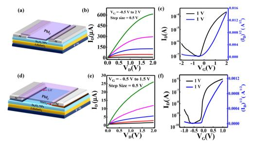
Fig. 6 (a) Schematic of Pbl<sub>2</sub>-coated Device-1, and its (b) output characteristics and (c) transfer characteristics. (d) Schematic of Pbl<sub>2</sub>-coated Device-2, and its (e) output characteristics and (f) transfer characteristics.
