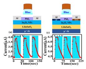
Fig. 10 Transient photoresponse of Pbl2-coated TFT under multiple cycle blue light illumination: (a) Device-1 (with symmetric S-D electrodes) and (b) Device-2 (with asymmetric S-D electrodes).
