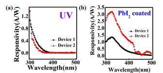
Fig. 12 Responsivity of Device-1 and Device-2: (a) without Pbl<sub>2</sub> layer and (b) with Pbl<sub>2</sub> layer (plotted from the EQE data).
