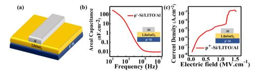
Fig. 4 (a) Schematic of the MIM device structure of p<sup>+</sup>-Si/LilnSnO<sub>4</sub>/Al. Electrical characterization of LilnSnO<sub>4</sub> dielectric film with MIM device. (b) Variation in capacitance with frequency and (c) variation in current density with applied field.
