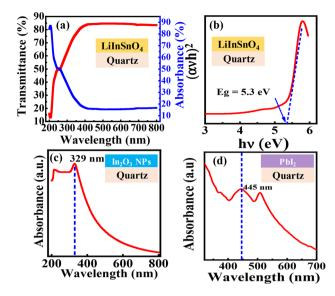
Fig. 2 (a) Optical transmittance/absorbance spectra of the solution-processed LilnSnO<sub>4</sub> dielectric thin film annealed at 550 °C for LilnSnO<sub>4</sub>/ quartz. (b) Tauc plot of LilnSnO<sub>4</sub>; the band gap is 5.3 eV. Absorbance spectra of (c)  $In_2O_3$  NPs and (d)  $Pbl_2$  thin films.
