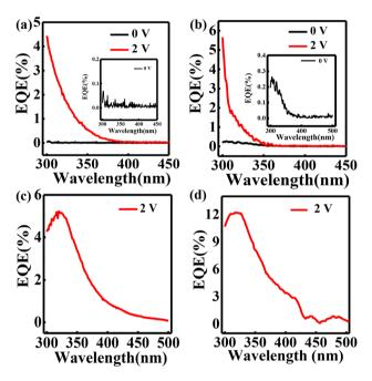
Fig. 11 External quantum efficiency at 0 V and 2 V without any additional Pbl<sub>2</sub> layer: (a) symmetric electrode TFT and (b) asymmetric electrode TFT. External Quantum efficiency with the PbI<sub>2</sub>-coated device at 2 V with (c) symmetric electrode and (d) asymmetric electrode TFTs.
