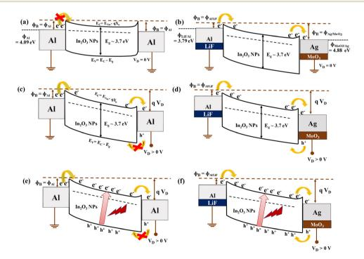
Fig. 13 Band diagram of (a) Device-1 and (b) Device-2 at equilibria with zero biasing ( $V_D = 0$  V), (c) Device-1 and (d) Device-2 under electrical biasing ( $V_D > 0$  V), and (e) Device-1 and (f) Device-2 under electrical ( $V_D > 0$  V) and optical illumination.
