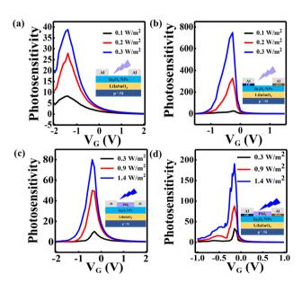
Fig. 8 Photosensitivity plot of TFTs under UV illumination with (a) symmetric electrode and (b) asymmetric electrode. Photosensitivity plot of Pbl2-coated TFTs under blue illumination with (c) symmetric electrode and (d) asymmetric electrode.
