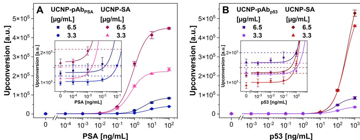
**Fig. 3** Calibration curves obtained using Er-doped UCNPs conjugated with polyclonal antibodies in ULISA for (A) PSA and (B) p53. Error bars represent the standard deviations of 3 independent wells. The dotted lines represent 3 times the standard deviation of the blank above the baseline of the regression curve, and their intersections with the respective fits correspond to the LODs.
