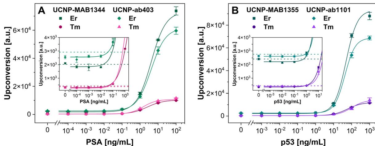
**Fig. 4** Calibration curves obtained using Er- and Tm-doped UCNPs conjugated with monoclonal antibodies in ULISA for (A) PSA and (B) p53. Error bars represent the standard deviations of 3 independent wells. The dotted lines represent 3 times the standard deviation of the blank above the baseline of the regression curve, and their intersections with the respective fits correspond to the LODs.
