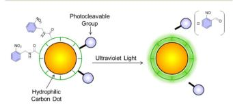
Fig. 1 Photoinduced uncaging and fluorescence activation of 2-nitrobenzyl carbon dots.
