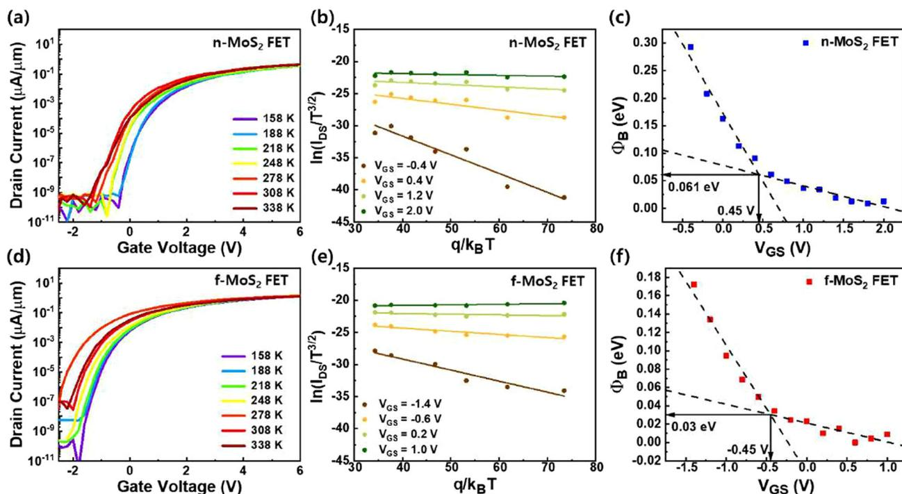
Fig. 5 Temperature-dependent  $I_D - V_G$  transfer curves of (a) the n-MoS<sub>2</sub> FET and (d) the f-MoS<sub>2</sub> FET from 158 to 338 K. Arrhenius plots of (b) the n-MoS<sub>2</sub> FET at gate voltages from -1.4 to 1.0 V and (e) the f-MoS<sub>2</sub> FET at  $V_G$  from -0.4 to 2.0 V. Extracted effective barrier heights ( $\phi_{SB}$ ) of (c) the n-MoS<sub>2</sub> FET and (f) the f-MoS<sub>2</sub> FET as a function of  $V_{GS}$ .
