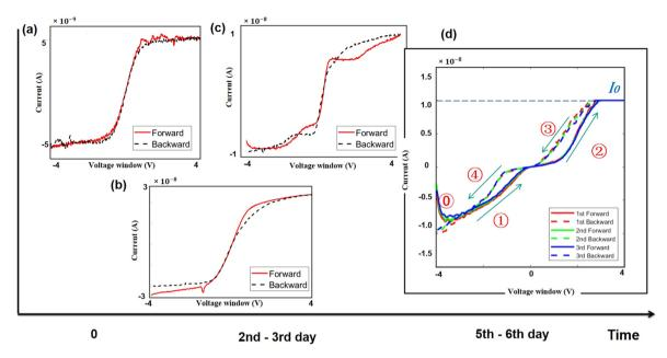
Fig. 2 I-V curve of (a) the brand new fabricated device and (b and c) the device gradually oxidized naturally, showing unpredictable and uncontrollable behaviour. (d) Repeated volatile hysteresis after five days; the oxidation process reaches an equilibrium state.
