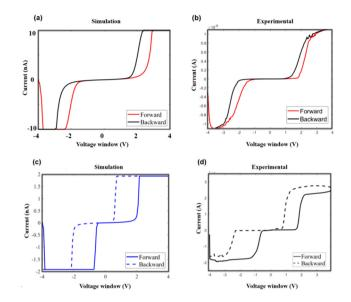
Fig. 10 The comparison of simulated and experimental data. (a) The simulation results with a higher saturation current. (b) A representative measured I/V curve with an annealed device, showing a higher saturation current and small hysteresis. (c) The simulation results with a lower saturation current. (d) A representative measured I/V curve of the device without annealing, showing a lower saturation current and greater hysteresis.
