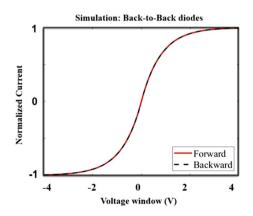
Fig. 9 The simulated current of pure back-to-back diodes.
