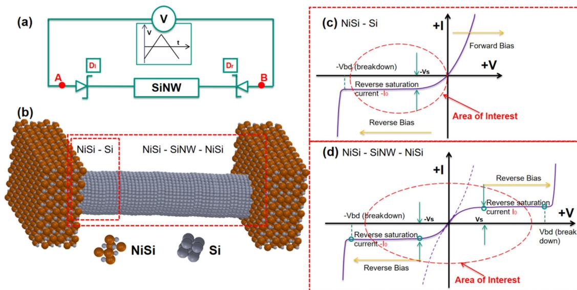
**Fig. 8** (a) Scheme of driving back-to-back Schottky diode structure with a triangular waveform signal. (b) Schematic of back-to-back Schottky diode structure formed across SiNW with a triangular signal. (c)  $I$ - $V$  characteristics of a single diode. (d)  $I$ - $V$  characteristics within a single voltage sweep through the back-to-back Schottky diode structure.
