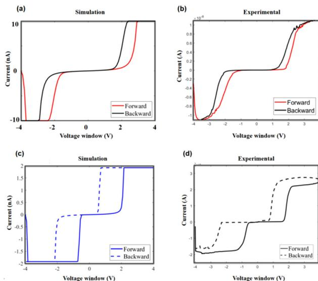
**Fig. 10** The comparison of simulated and experimental data. (a) The simulation results with a higher saturation current. (b) A representative measured  $I/V$  curve with an annealed device, showing a higher saturation current and small hysteresis. (c) The simulation results with a lower saturation current. (d) A representative measured  $I/V$  curve of the device without annealing, showing a lower saturation current and greater hysteresis.
