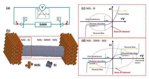
Fig. 8 (a) Scheme of driving back-to-back Schottky diode structure with a triangular waveform signal. (b) Schematic of back-to-back Schottky diode structure formed across SiNW with a triangular signal. (c) *I–V* characteristics of a single diode. (d) *I–V* characteristics within a single voltage sweep through the back-to-back Schottky diode structure.
