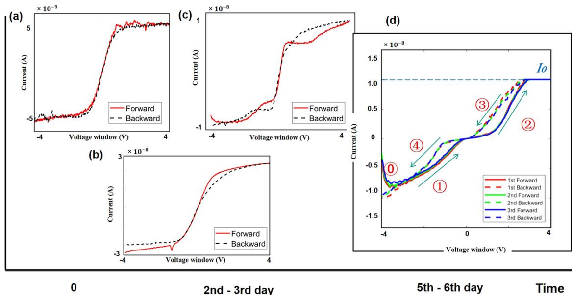
Fig. 2  $I$ - $V$  curve of (a) the brand new fabricated device and (b and c) the device gradually oxidized naturally, showing unpredictable and uncontrollable behaviour. (d) Repeated volatile hysteresis after five days; the oxidation process reaches an equilibrium state.
