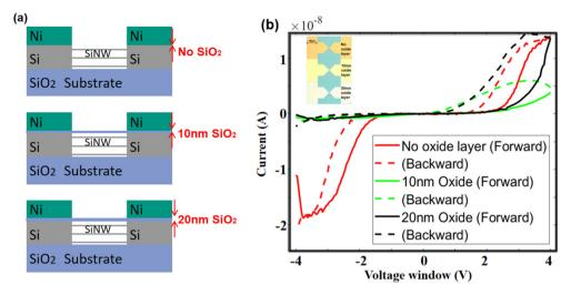
Fig. 7 (a) Schematic of the intermediate oxide layer. (b) Memristive behaviour with different thicknesses of different intermediate oxide layers.
