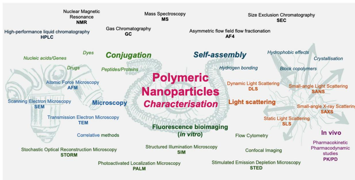
Fig. 1 Summary of polymer and polymer nanoparticle characterisation methods.
