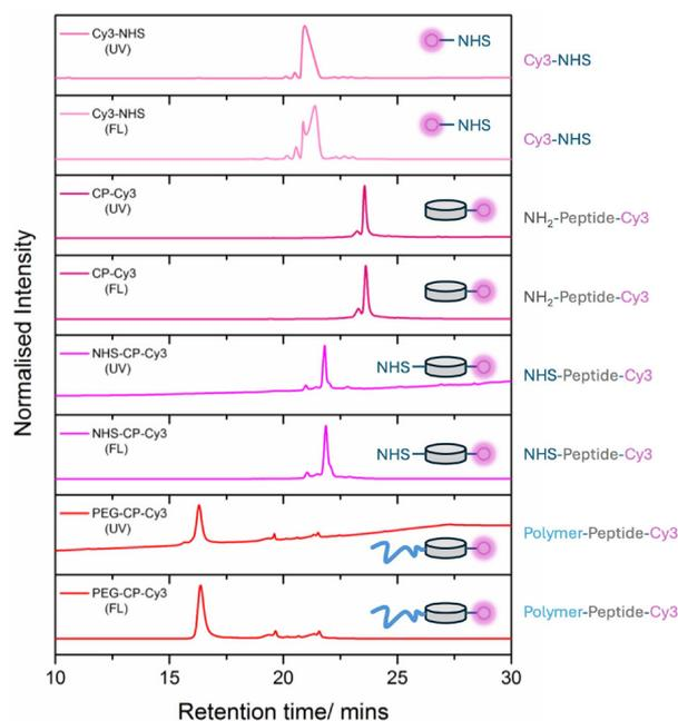
**Fig. 2** High-performance liquid chromatography (HPLC) of peptide-polymer-dye conjugate. UV absorption at 280 nm (tryptophan absorption to follow the peptide), fluorescence emission measured at 570 nm upon excitation at 555 nm (to follow the Cyanine 3 dye). Adapted from Rho *et al.*, reproduced with permission from Wiley.<sup>88</sup>
