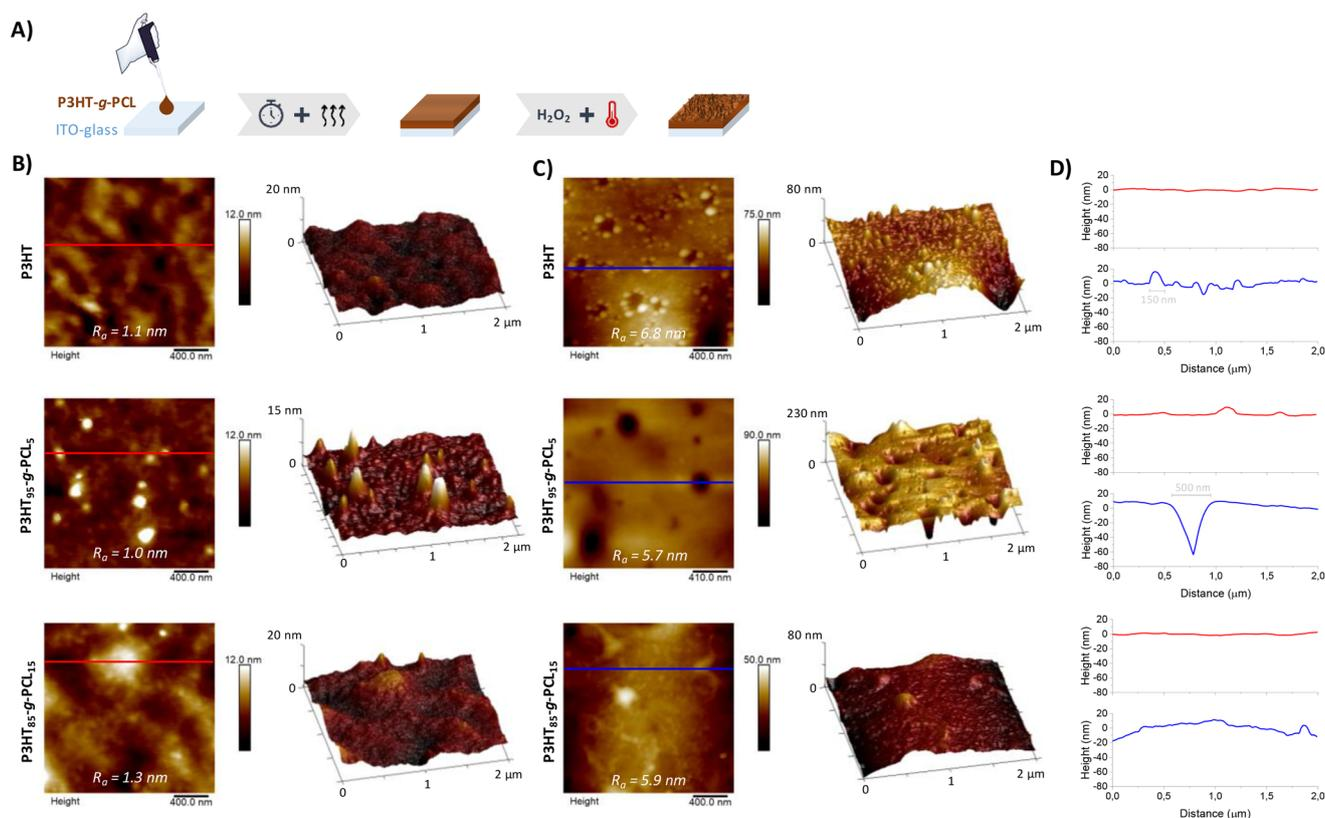
**Fig. 2** (A) Schematic representation of the fabrication of the films, followed by a thermo-oxidative step. (B) 2D (left) and 3D (right) topographical AFM images of the thin films before thermo-oxidation. (C) 2D (left) and 3D (right) topographical AFM images of the thin films after thermo-oxidation. Red and blue lines show the cut-positions to determine the pore dimensions in (D).
