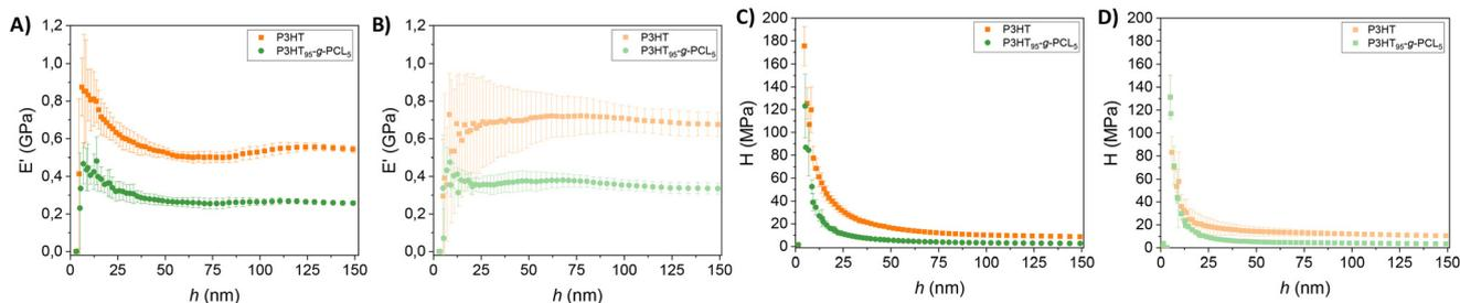
Fig. 3 Storage modulus ( $E'$ ) of the P3HT and P3HT<sub>95-g</sub>-PCL<sub>5</sub> films (A) before and (B) after the thermo-oxidative process. Hardness ( $H$ ) of the P3HT and P3HT<sub>95-g</sub>-PCL<sub>5</sub> films (C) before and (D) after the thermo-oxidative process.
