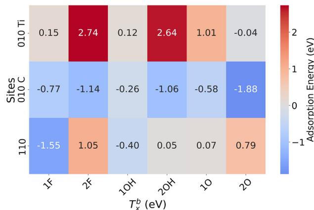
**Fig. 6** Most stable adsorption energies of single hydrogen adsorbed on the  $\{010\}$  C,  $\{010\}$  Ti, and  $\{110\}$  edge sites of  $\text{Ti}_2\text{CO}_2$ , i.e., ( $\text{T}_x^{\text{b}} = \text{O}$ ), with different edge terminations  $\text{T}_x^{\text{e}} = 1$  ML F, 2 ML F, 1 ML OH, 2 ML OH, 1 ML O, or 2 ML O.
