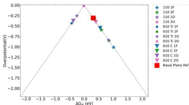
**Fig. 7** HER volcano plot with computational overpotentials of  $Ti_2CO_2$  for the 3 types of edges considered and their various terminations:  $T_x^e = O, OH,$  and  $F$  at 1 and 2 ML coverages.
