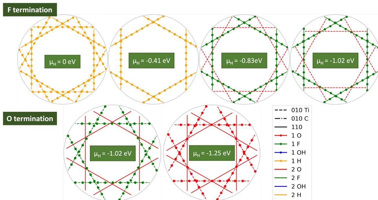
**Fig. 5** Wulff constructions of  $\text{Ti}_2\text{CT}_x$  at different chemical potentials where the dominating termination changes from F to O at  $\mu_{\text{H}} = -1$  eV. These results are based on the results from the basal plane and edge termination stability analysis.
