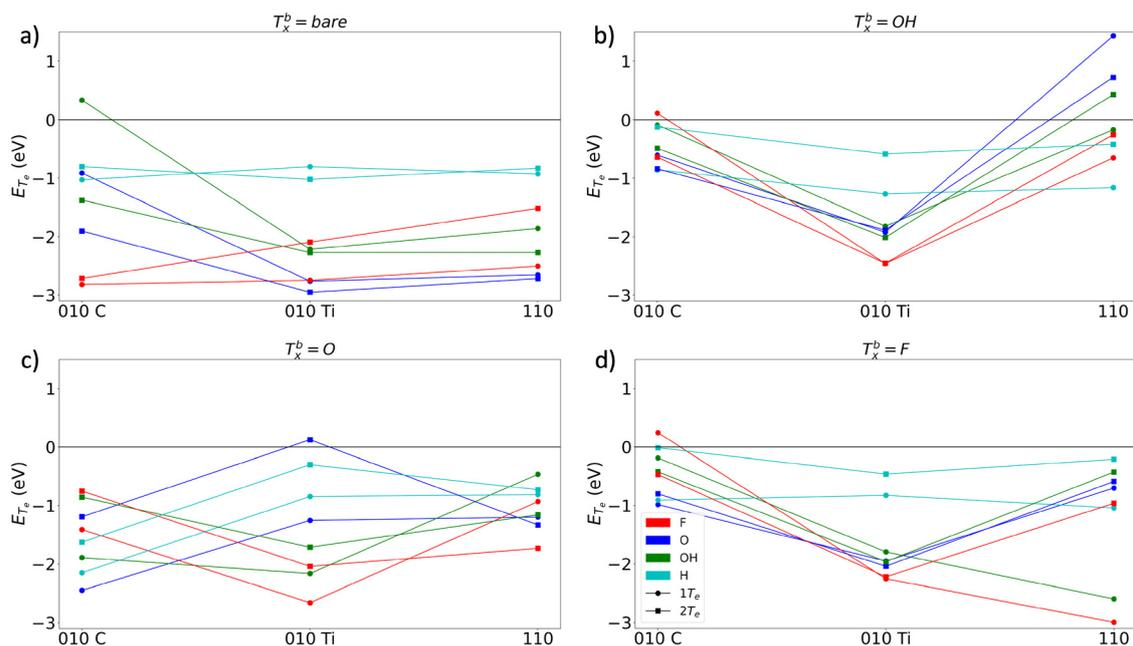
**Fig. 2** Calculated adsorption energy normalized per adsorbate  $E_{T_x^e}$  of the edge terminations (O, F, and OH) of the {010} C, {010} Ti and {110} MXene NRs as a function of different basal plane terminations ( $T_x^b$ ) being (a) bare basal plane, (b)  $T_x^b = \text{OH}$ , (c)  $T_x^b = \text{O}$ , and (d)  $T_x^b = \text{F}$ .
