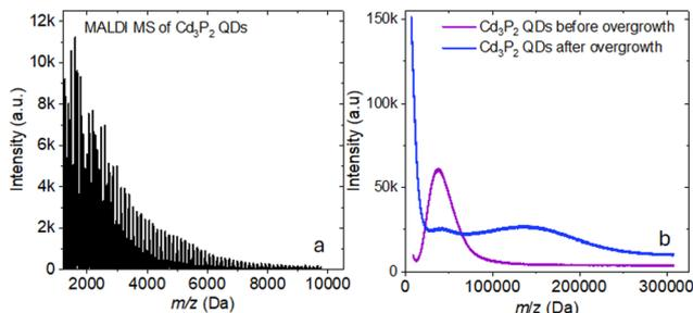
**Fig. 5** (a) MALDI MS of  $\text{Cd}_3\text{P}_2$  QDs emitting at 1010 nm in the low-mass region before cluster overgrowth. (b) MALDI MS of  $\text{Cd}_3\text{P}_2$  QDs in the high-mass region before and after cluster overgrowth.
