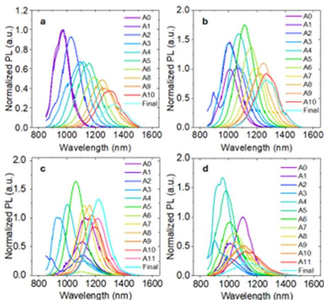
**Fig. 3** PL spectra of the aliquots of continuous injection of cadmium phosphide clusters on  $\text{Cd}_3\text{P}_2$  QDs initially emitting at: (a) 965 nm, (b) 1010 nm, (c) 1102 nm, (d) 1145 nm.
