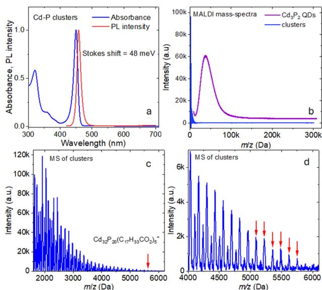
**Fig. 1** (a) Absorption and PL spectra of cadmium phosphide magic-sized clusters (MSCs). (b) MALDI mass-spectra of Cd<sub>3</sub>P<sub>2</sub> QDs and the MSCs in the high-mass region (c) MALDI MS of the MSCs in the region from 2000 to 6000 Da. The composition of the heaviest identifiable fragment is indicated (d) MALDI MS of the MSCs in the region from 4000 to 6000 Da. The arrows point to the heaviest identifiable fragment peaks.
