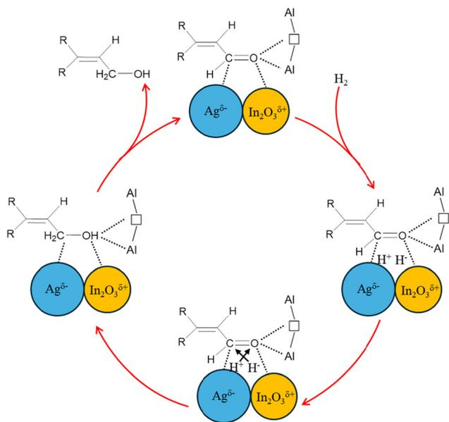
Fig. 4 The proposed mechanism for the hydrogenation of UALs to UOLs over Ag-In<sub>2</sub>O<sub>3</sub>/f-m-Al<sub>2</sub>O<sub>3</sub>.
