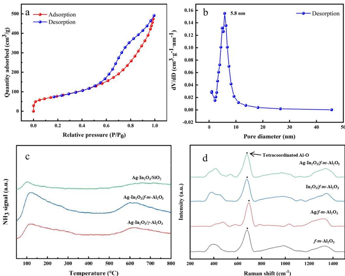
Fig. 3 (a)  $\text{N}_2$  adsorption–desorption isotherm. (b) Pore size distribution diagram of the  $\text{Ag-In}_2\text{O}_3/f\text{-}m\text{-Al}_2\text{O}_3$  catalyst. (c)  $\text{NH}_3$ -TPD of different catalysts. (d) Raman spectra for different catalysts.
