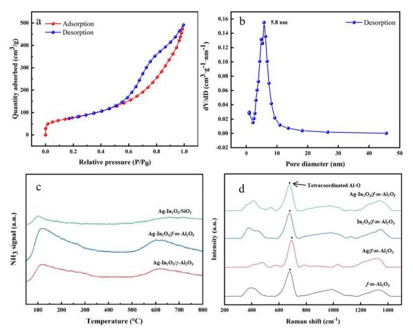
Fig. 3 (a) N<sub>2</sub> adsorption-desorption isotherm. (b) Pore size distribution diagram of the Ag-In<sub>2</sub>O<sub>3</sub>/f-m-Al<sub>2</sub>O<sub>3</sub> catalyst. (c) NH<sub>3</sub>-TPD of different catalysts. (d) Raman spectra for different catalysts.
