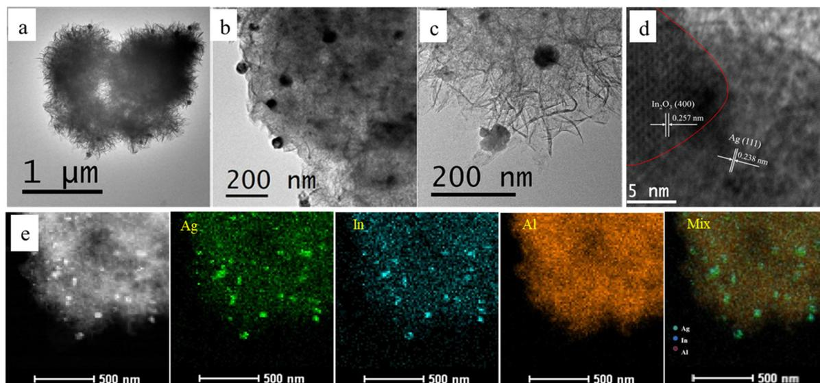
**Fig. 1** (a), (b) and (c) Transmission electron microscopy images of Ag–In<sub>2</sub>O<sub>3</sub>/f-*m*-Al<sub>2</sub>O<sub>3</sub> at different magnifications. (d) High resolution transmission electron microscopy image of Ag–In<sub>2</sub>O<sub>3</sub>/f-*m*-Al<sub>2</sub>O<sub>3</sub>. (e) STEM-HAADF image of Ag–In<sub>2</sub>O<sub>3</sub>/f-*m*-Al<sub>2</sub>O<sub>3</sub> and mapping images of Ag, In, and Al elements and their overlap.
