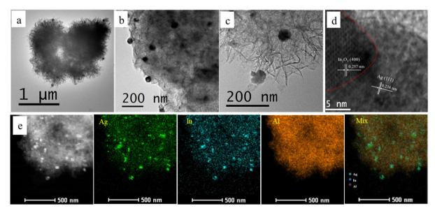
Fig. 1 (a), (b) and (c) Transmission electron microscopy images of Ag-In<sub>2</sub>O<sub>3</sub>/f-m-Al<sub>2</sub>O<sub>3</sub> at different magnifications. (d) High resolution transmission electron microscopy image of Aq-In<sub>2</sub>O<sub>3</sub>/f-m-Al<sub>2</sub>O<sub>3</sub>. (e) STEM-HAADF image of Aq-In<sub>2</sub>O<sub>3</sub>/f-m-Al<sub>2</sub>O<sub>3</sub> and mapping images of Aq, In, and Al elements and their overlap.
