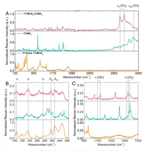
Fig. 2 (A) Normalized Raman spectra of pristine 1T-MoS<sub>2</sub>, ChNH<sub>2</sub>, and 1T-MoS<sub>2</sub>-ChNH<sub>2</sub>; (B) magnification of the region comprised between 140 and 490 cm<sup>-1</sup>; (C) magnification of the region comprised between 950 and 1550 cm<sup>-1</sup>. All spectra were collected using a 633 nm excitation source.
