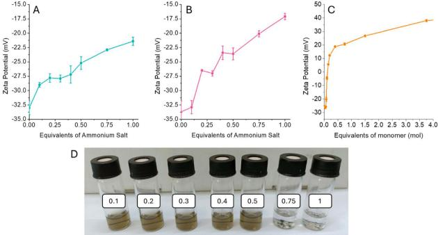
Fig. 1 Zeta potential titration of 1T-MoS<sub>2</sub> with ChNH<sub>2</sub> (A), Et<sub>x</sub>NEtNH<sub>2</sub> (B), and polyDADMAC (C). (D) Photograph of 1T-MoS<sub>2</sub> suspensions with the addition of 0.1, 0.2, 0.3, 0.4, 0.5, 0.75 and 1 equivalent of ChNH<sub>2</sub>.
