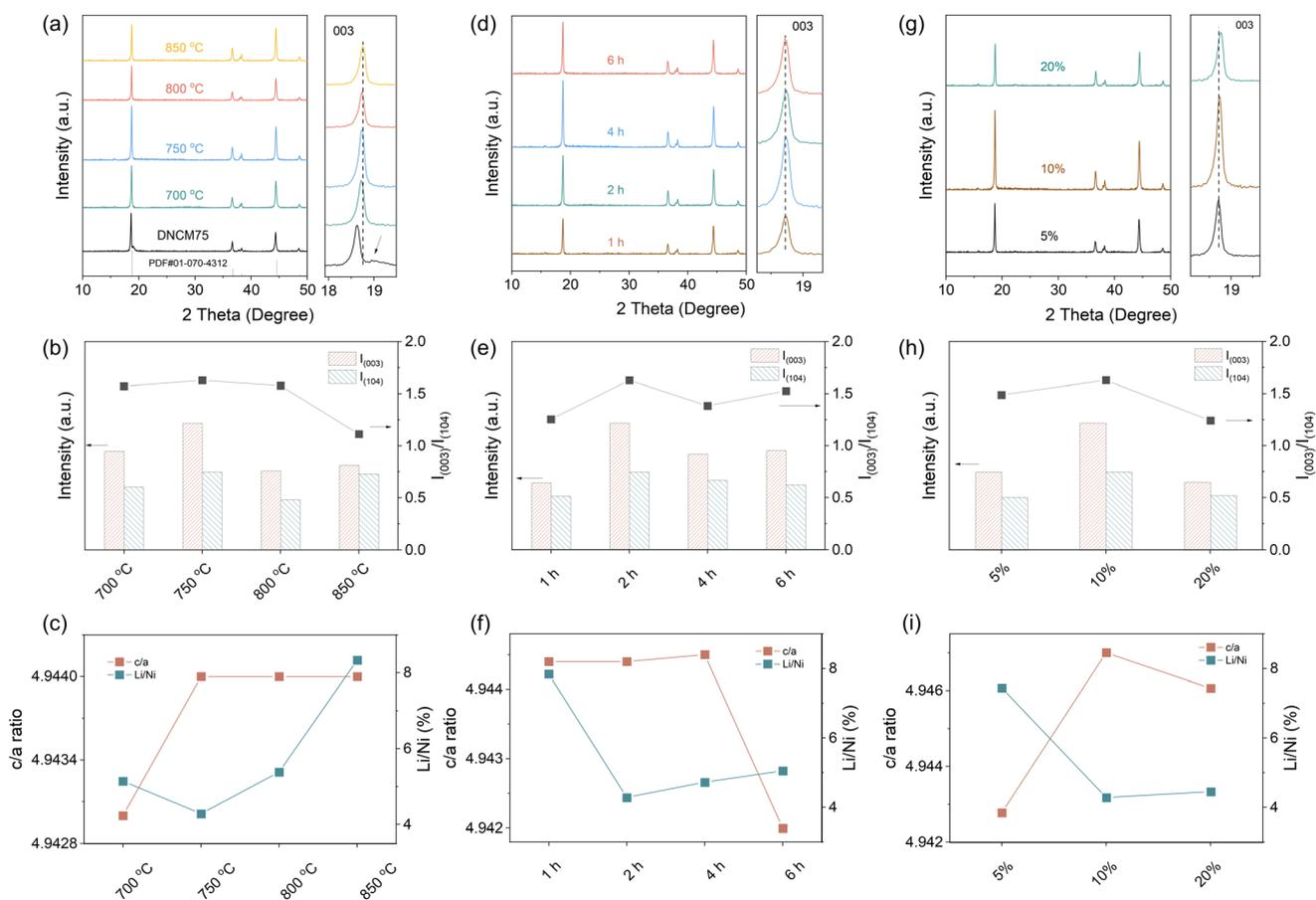
**Fig. 2** (a) XRD patterns, (b)  $I_{(003)}/I_{(104)}$  ratios and (c)  $c/a$  ratios and Li/Ni mixing of RNCM70 sintered at 700 °C, 750 °C, 800 °C, and 850 °C; (d) XRD patterns, (e)  $I_{(003)}/I_{(104)}$  ratios and (f)  $c/a$  ratios and Li/Ni mixing of RNCM70 sintered at 750 °C for 1, 2, 4, and 6 hours; (g) XRD patterns, (h)  $I_{(003)}/I_{(104)}$  ratios and (i)  $c/a$  ratios and Li/Ni mixing of RNCM70 sintered at 750 °C with 5%, 10%, and 20% excess Li<sub>2</sub>CO<sub>3</sub>.
