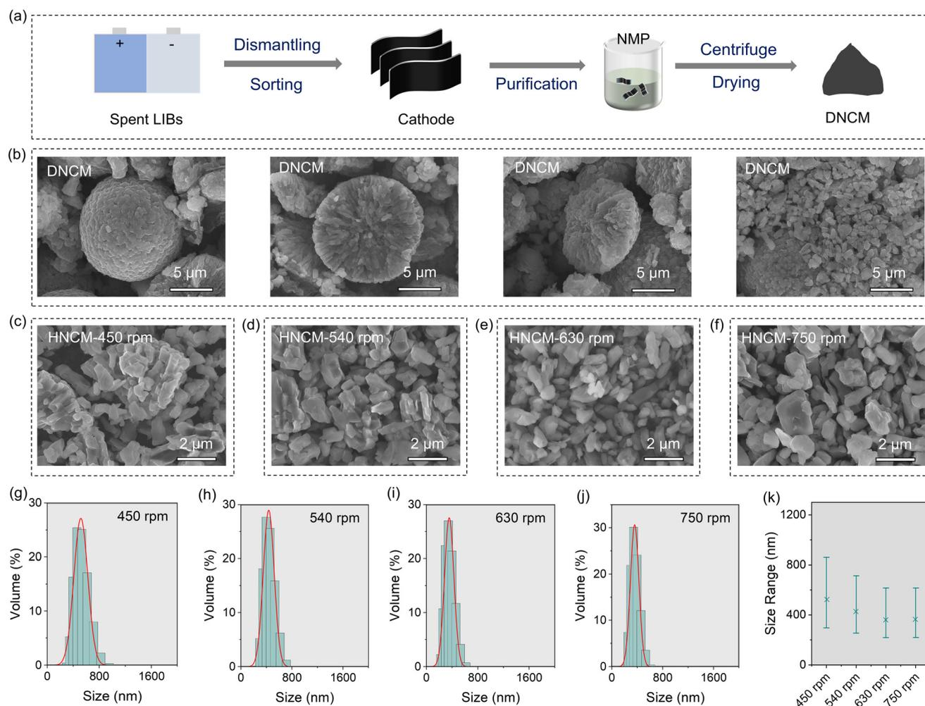
**Fig. 1** (a) Schematic illustration of the disassembly process of the waste NCM70 battery; (b) SEM images of DNCM70; (c–f) SEM images of HDNCM70 milled at 450, 540, 630, and 750 rpm; (g–j) DLS results of HDNCM70 milled at different speeds, with the corresponding size distribution summarized in (k).
