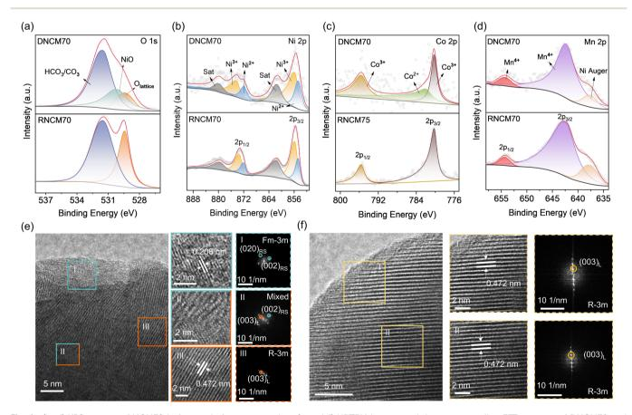
Fig. 4 (a-d) XPS spectra of NCM70 before and after regeneration; (e and f) HRTEM images and the corresponding FFT patterns of DNCM70 and
