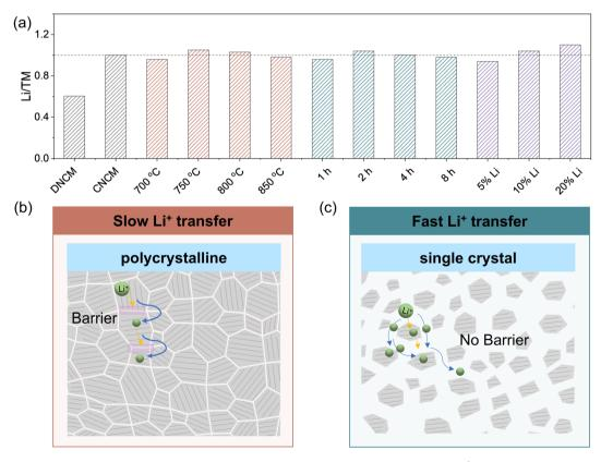
Fig. 3 (a) The Li contents in RNCM70 under different conditions; (b and c) schematic illustration of the Li<sup>+</sup> diffusion pathway in polycrystalline and single-crystalline NCM particles.
