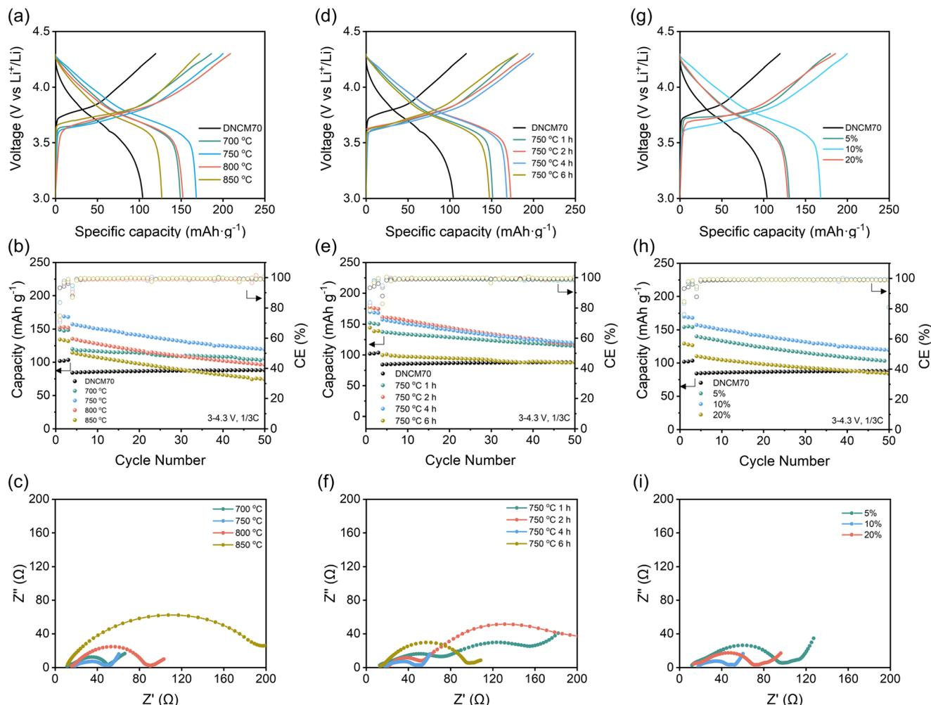
**Fig. 5** (a–c) Voltage profiles, cycling performance and Nyquist plots of RNCM70 sintered at 700 °C, 750 °C, 800 °C, and 850 °C; (d–f) voltage profiles, cycling performance and Nyquist plots of RNCM70 sintered at 750 °C for 1, 2, 4, and 6 hours; (g–i) voltage profiles, cycling performance and Nyquist plots of RNCM70 sintered at 750 °C with 5%, 10%, and 20% excess  $\text{Li}_2\text{CO}_3$ .
