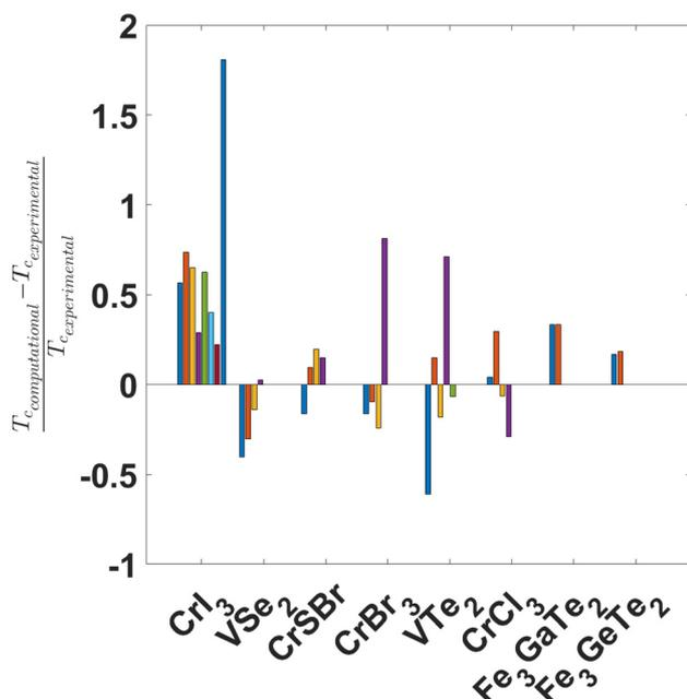
**Fig. 13** Comparison of calculated critical temperatures of 2D magnets with the experimental value. The data shown comes from Table 5. Since we are not aware of any experimental estimation of the critical temperature of  $\text{VTe}_2$ , we take its value as the mean from those in Table 5.
