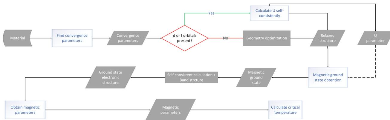
**Fig. 11** Sketch of the workflow to follow when modelling 2D magnetic materials from DFT to the calculation of their critical temperature. All the steps in this workflow are covered throughout this review paper.
