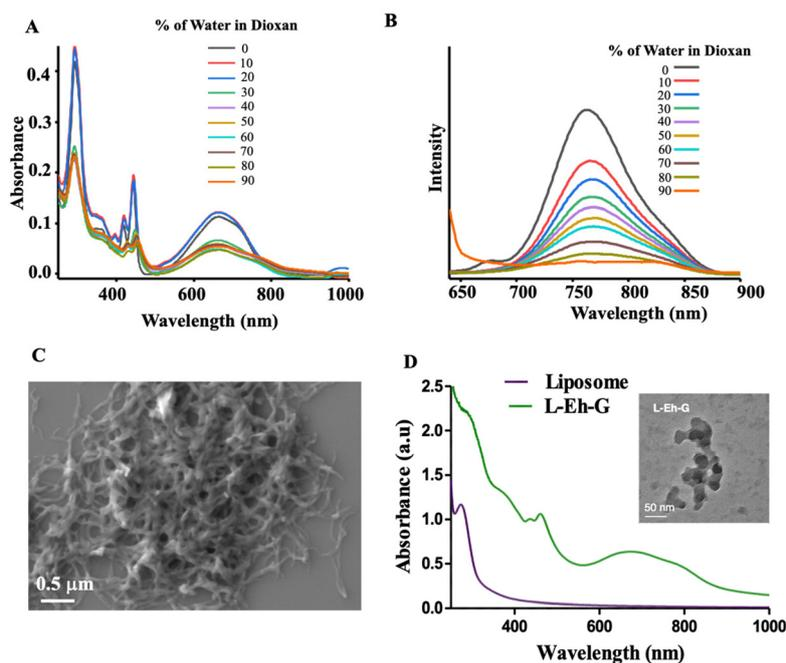
**Fig. 1** A. Absorption spectra of Eh-G at different vol% of water in dioxane. B. Emission spectra of Eh-G at different vol% of water in dioxane ( $\lambda_{\text{exc}} = 620$  nm). C. FE-SEM image of Eh-G in 90 vol% water in dioxane. D. Absorption spectra of plain liposomes and liposomes encapsulated with Eh-G (L-Eh-G). The TEM image of L-Eh-G is shown in the inset of D.
