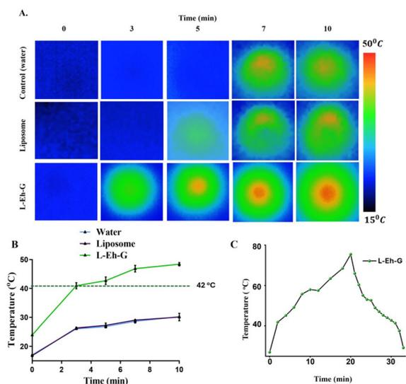
**Fig. 3** A. Thermal images of control (Millipore water), free liposomes, and L-Eh-G nanoformulations. B. Photothermal heating curves of control (Millipore water), free liposome and L-Eh-G nanoformulations under 750 nm laser irradiation. C. The heating and cooling curves of L-Eh-G.
