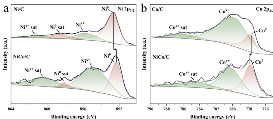
Fig. 2 (a) Ni 2p<sub>3/2</sub> core-level XPS spectra of Ni/C and NiCo/C. (b) Co 2p<sub>3/2</sub> core-level XPS spectra of Co/C and NiCo/C.
