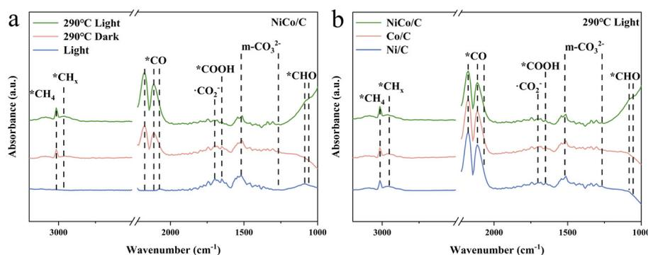
**Fig. 4** (a) *In situ* DRIFTS spectra of the NiCo/C catalyst under solely light-driven, thermal catalytic (at 290 °C in dark), and photo-thermal conditions for 60 min. (b) *In situ* DRIFTS spectra of Ni/C, Co/C and NiCo/C catalysts at 290 °C under light irradiation for 60 min.
