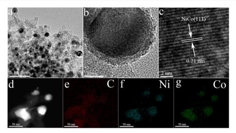
Fig. 1 (a) TEM images of NiCo/C. (b) and (c) HRTEM images of NiCo/C. (d) HAADF-STEM images of NiCo/C. EDS mapping images of (e) C, (f) Ni and (g) Co for NiCo/C.
