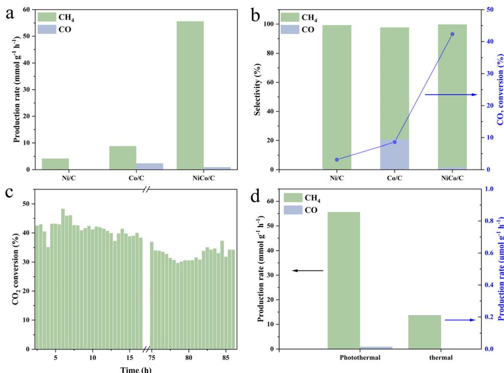
**Fig. 3** (a) Production rate of CH<sub>4</sub> and CO of Ni/C, Co/C and NiCo/C catalysts at 290 °C under light irradiation. (b) Product selectivities and CO<sub>2</sub> conversion rates of Ni/C, Co/C and NiCo/C catalysts at 290 °C under light irradiation. (c) Production rates of CH<sub>4</sub> and CO of the NiCo/C catalyst under different conditions. (d) CO<sub>2</sub> conversion of the NiCo/C catalyst during long-time reaction at 290 °C under light irradiation.
