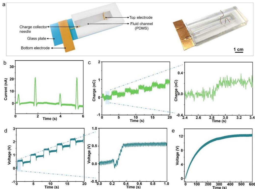
**Fig. 1** The device structure and output performance of the triboelectric charge-separable probe (the type of droplet is deionized water). (a) Schematic diagram and image of the device structure. (b) Variation of device output current over time. (c) Characterization of device transferred charge. (d) and (e) Output voltage signal of the device.
