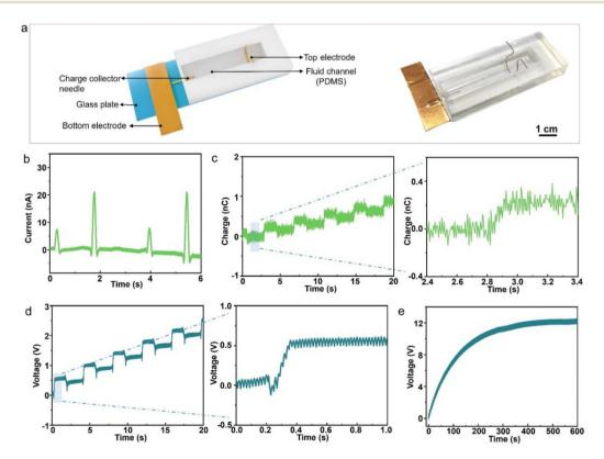
Fig. 1 The device structure and output performance of the triboelectric charge-separable probe (the type of droplet is deionized water). (a) Schematic diagram and image of the device structure. (b) Variation of device output current over time. (c) Characterization of device transferred charge. (d) and (e) Output voltage signal of the device.
