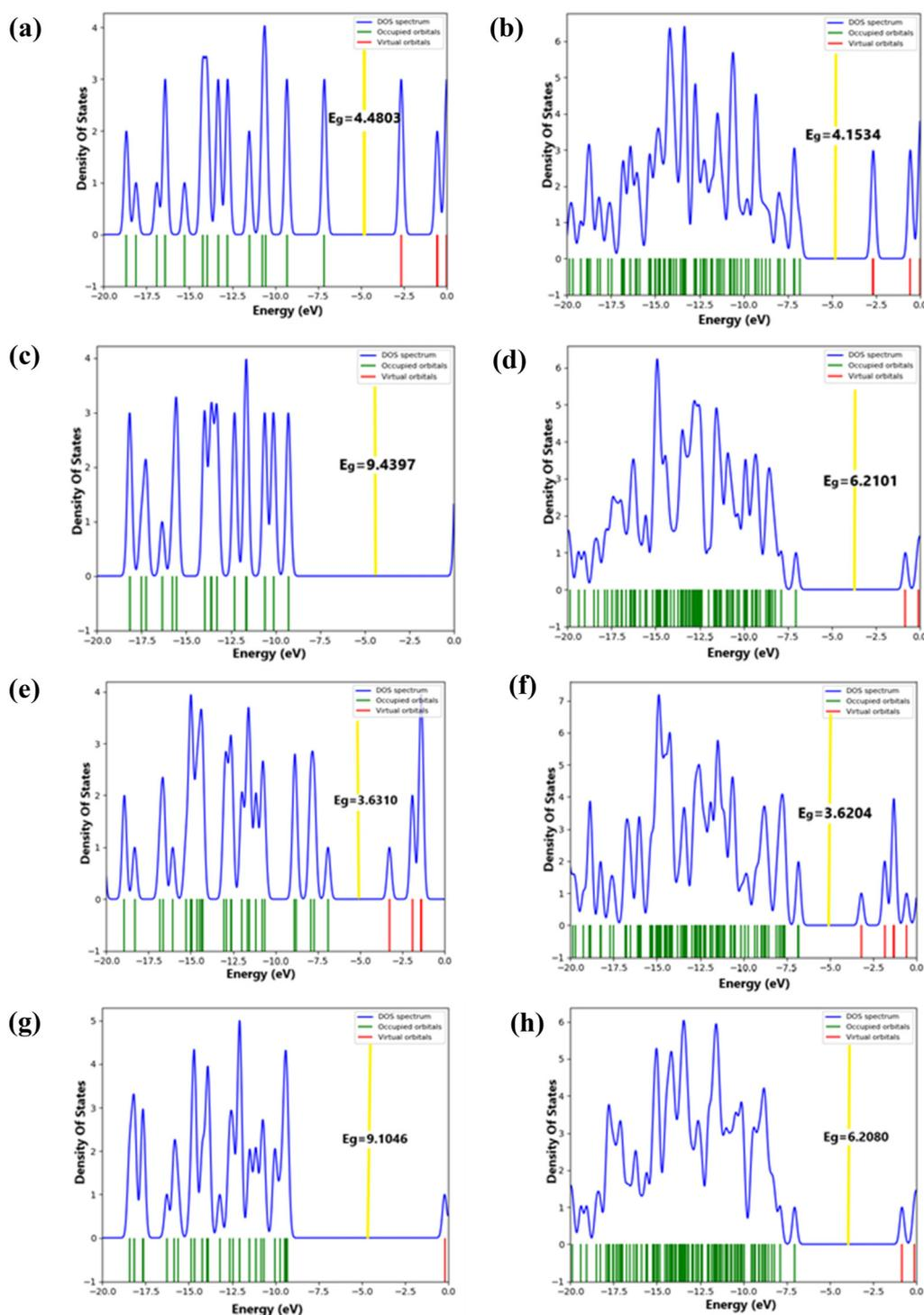
**Fig. 3** (a) DOS spectra of the  $C_{24}$  nanocage, (b) methyl erlotinib@ $C_{24}$  nanocage, (c)  $B_{12}N_{12}$  nanocage, (d) methyl erlotinib@ $B_{12}N_{12}$  nanocage, (e)  $C_{32}$  nanocage, (f) methyl erlotinib@ $C_{32}$  nanocage, (g)  $B_{16}N_{16}$  nanocage, and (h) methyl erlotinib@ $B_{16}N_{16}$  nanocage. The Fermi level is represented by yellow.
