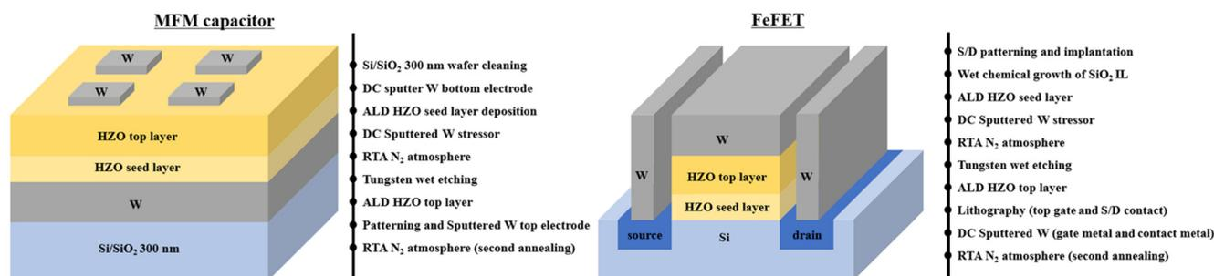
Fig. 1 Fabrication process flow and the schematic of an MFM capacitor and FeFET using the SPE method.
