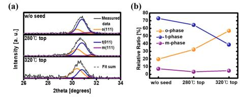
Fig. 4 (a) GI-XRD pattern in the  $2\theta$  range from 26° to 34° and (b) relative ratio of the phases of HZO films with and without SPE.
