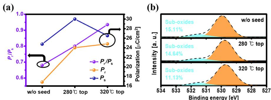
Fig. 7 (a) The relationship between  $P_r$  and  $P_s$  values in devices with and without SPE. (b) The sub-oxide (oxygen vacancy) ratio in the XPS spectra of O 1s for each device.
