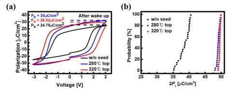
Fig. 5 (a) P-V hysteresis loops of 9 nm HZO FeCAPs, highlighting the effects of applying SPE and varying the deposition temperature of the top layer. (b) Device-to-device variation of each device.
