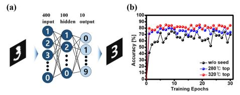
(a) Schematic of the 2-layer MLP neural network. (b) The inference accuracy for the MNIST handwritten digit image with and without SPE FeFETs.
