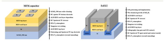
Fig. 1 Fabrication process flow and the schematic of an MFM capacitor and FeFET using the SPE method.
