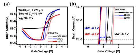
Fig. 6 (a)  $I_{\rm d}$  – $V_{\rm g}$  characteristics and (b) extracted MW with and without the SPE method of HZO-based FeFETs.
