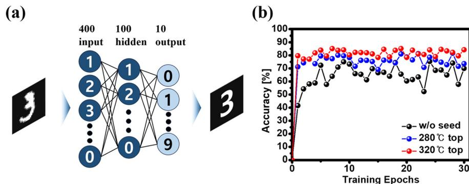
**Fig. 10** (a) Schematic of the 2-layer MLP neural network. (b) The inference accuracy for the MNIST handwritten digit image with and without SPE FeFETs.
