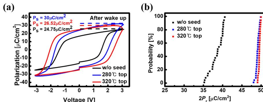
Fig. 5 (a)  $P$ - $V$  hysteresis loops of 9 nm HZO FeCAPs, highlighting the effects of applying SPE and varying the deposition temperature of the top layer. (b) Device-to-device variation of each device.
