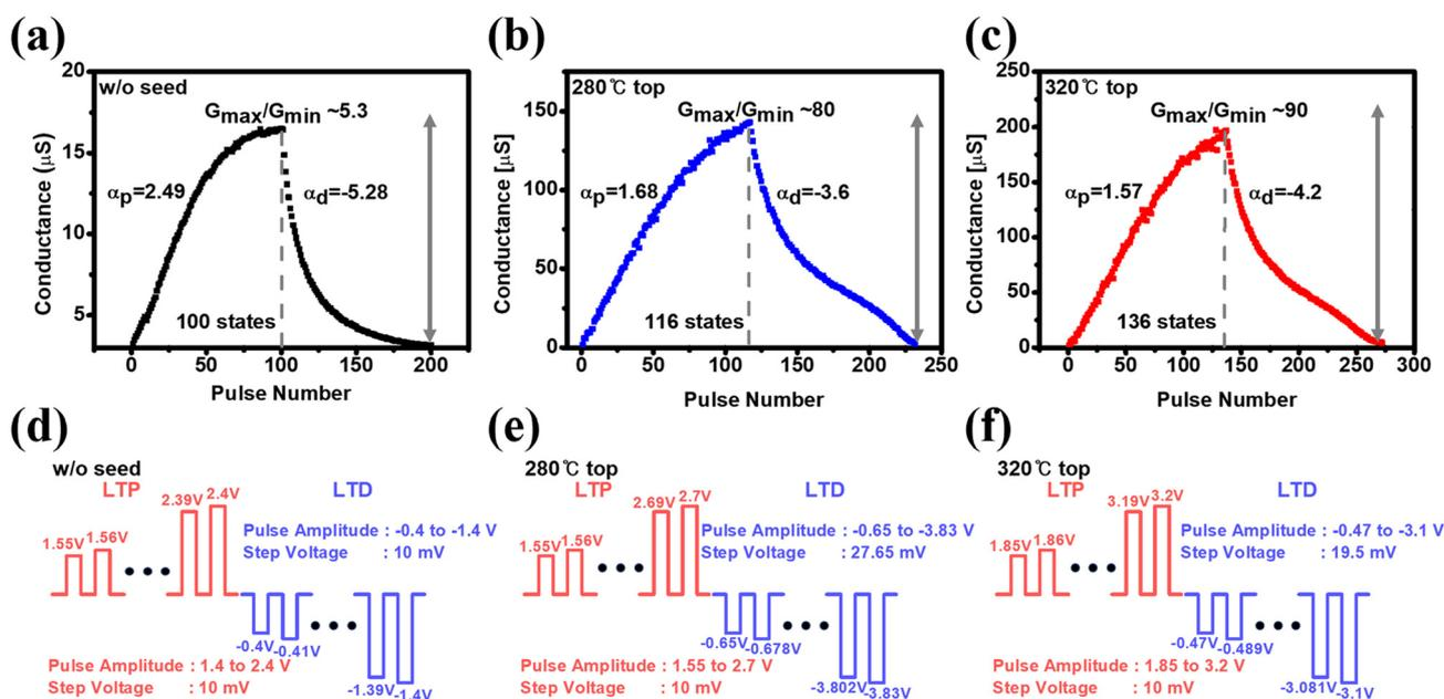
Fig. 9 LTP/LTD synaptic characteristics of: (a) FeFET without a seed layer, (b) top layer deposited at  $280$  °C with SPE and (c) top layer deposited at  $320$  °C with SPE FeFETs. (d)–(f) Schematic of potentiation/depression incremental pulse waveform.
