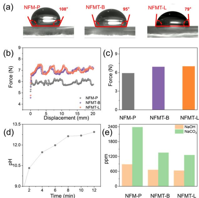
**Fig. 4** (a and b) Contact angle measurements of cathodes; (b) electrode detachment distance and adhesion force; (c) average adhesion force during electrode detachment; (d) pH variation of NFM-P in water over time; and (e) quantitative titration of  $\text{Na}_2\text{CO}_3$  and NaOH in NFM-P, NFMT-B, and NFMT-L.
