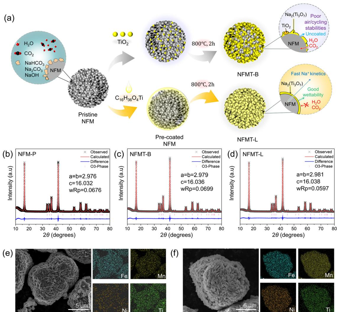
**Fig. 1** (a) Schematic illustration of the cathode materials' synthesis process; Rietveld refinement patterns of the XRD data for (b) NFM-P, (c) NFMT-B, and (d) NFMT-L; and SEM images and EDS results of (e) NFMT-B and (f) NFMT-L cathode materials.
