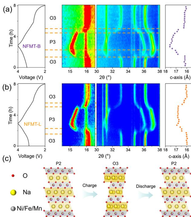
**Fig. 5** *In situ* XRD patterns of (a) NFMT-B and (b) NFMT-L during the first cycles and the corresponding lattice parameter changes; and (c) schematic diagram of the changes that occur in the crystal structure.
