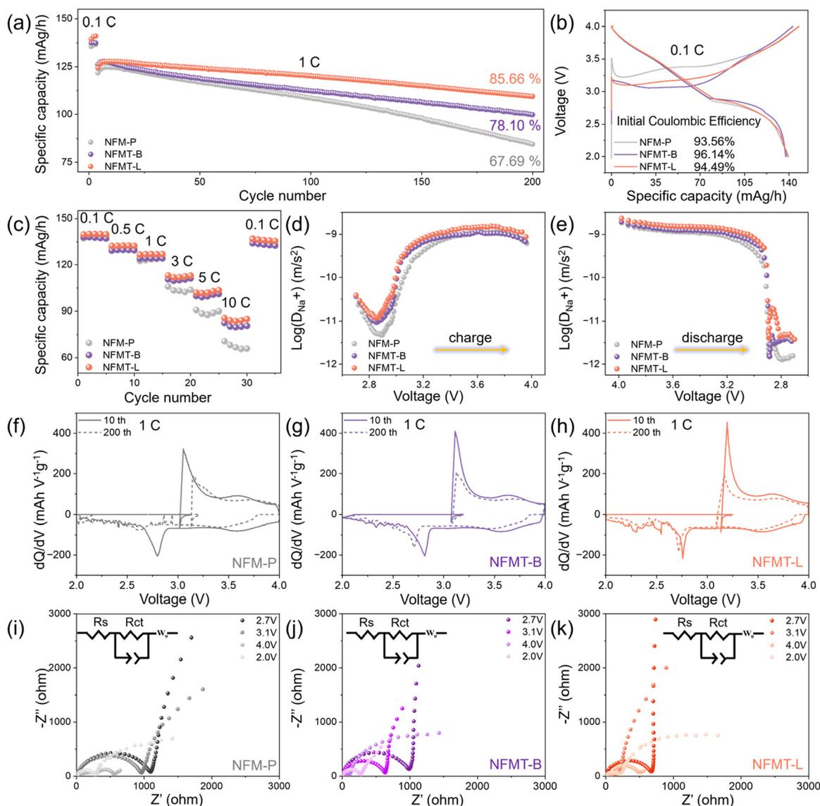
**Fig. 6** (a) Cycling performance; (b) the first charge/discharge curve at 12 mA h g<sup>-1</sup>; (c) rate performance; (d and e) GITT-calculated diffusion coefficients ( $D_{\text{Na}^+}$ ) of NFM-P, NFMT-B and NFMT-L; (f–h) dQ/dV curves after the 10th and 200th cycles; and (i–k) *in situ* EIS Nyquist plots at different potentials of NFM-P/NFMT-B/NFMT-L.
