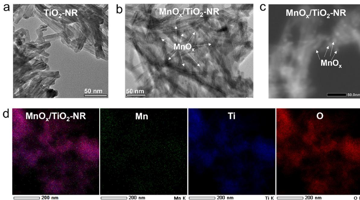
**Fig. 3** Bright field TEM images of (a)  $\text{TiO}_2$ -NR and (b)  $\text{MnO}_x/\text{TiO}_2$ -NR catalysts. (c) Dark-field image of the  $\text{MnO}_x/\text{TiO}_2$ -NR catalyst. (d) STEM-EDAX elemental mapping images of the  $\text{MnO}_x/\text{TiO}_2$ -NR catalyst.
