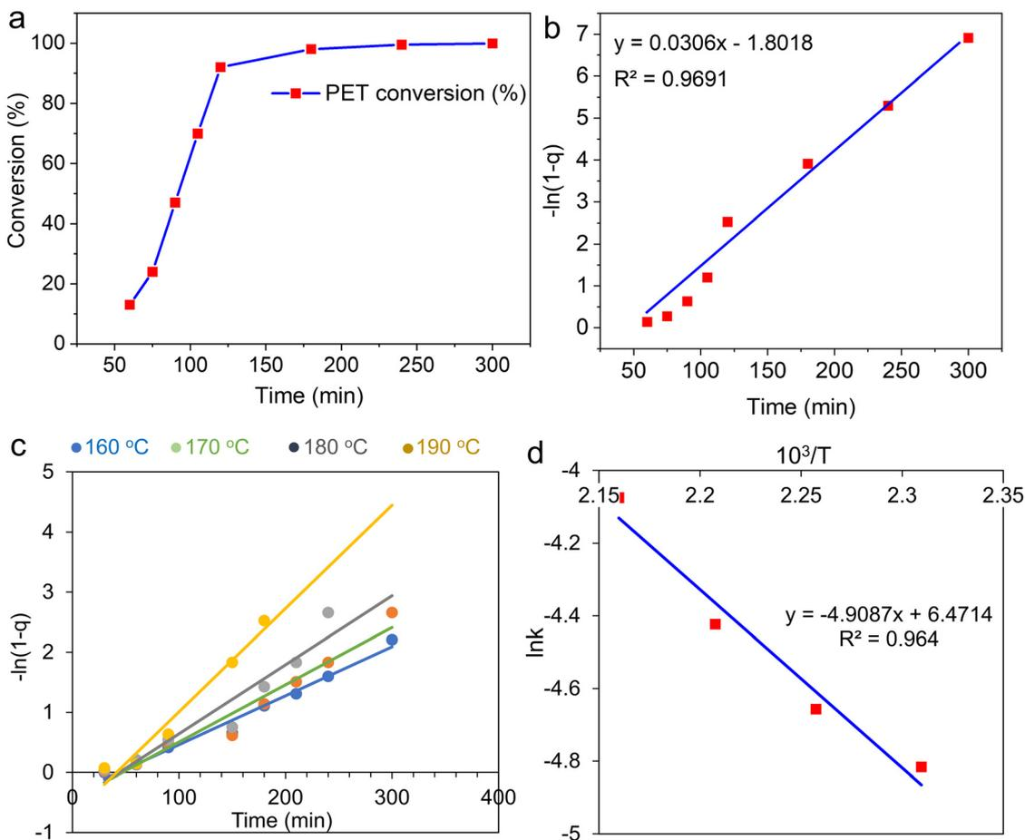
**Fig. 8** (a) PET conversion with the reaction time, (b) the plot of  $-\ln(1-q)$  with the reaction time ( $q = 1 - C_P/C_{P0}$ ), (c) conversion of PET at different temperatures and time intervals, and (d) Arrhenius plot of the PET glycolysis reaction over the  $\text{MnO}_x/\text{TiO}_2$ -NR catalyst.
