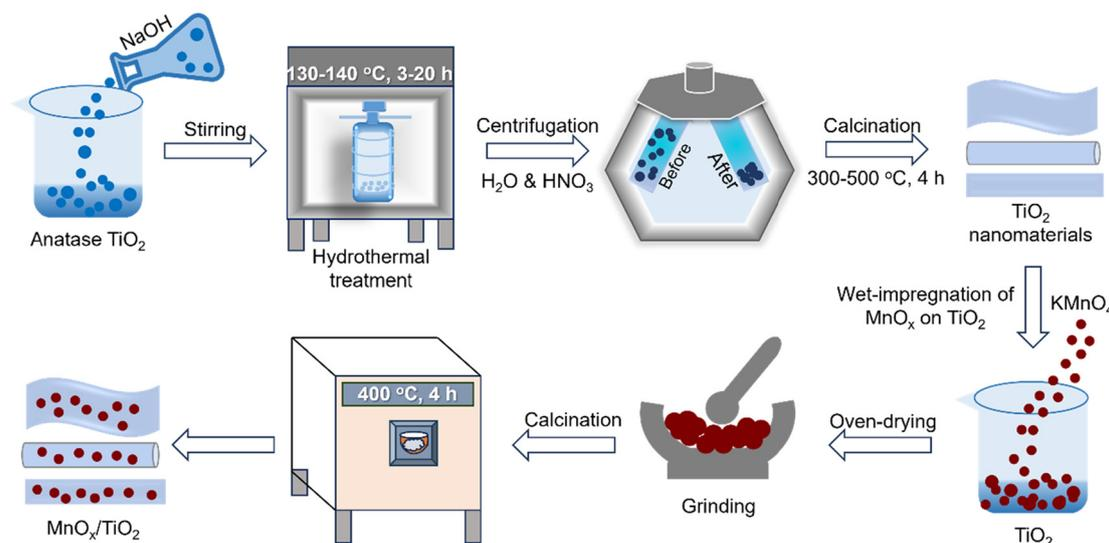
Fig. 2 The synthesis procedure of TiO<sub>2</sub> and MnO<sub>x</sub>/TiO<sub>2</sub> nanocatalysts.
