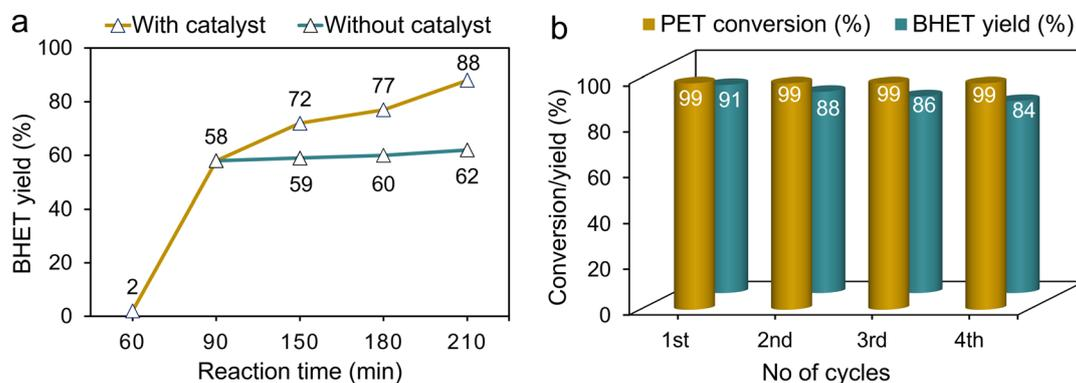
**Fig. 9** (a) Hot filtration test of the  $\text{MnO}_x/\text{TiO}_2$ -NR catalyst for PET glycolysis (reaction conditions: 1:20 molar ratio of PET:EG, 5 wt%  $\text{MnO}_x/\text{TiO}_2$ -NR catalyst, 190 °C, and 3 h). (b) Reusability studies (reaction conditions: 1:20 molar ratio of PET:EG, 5 wt%  $\text{MnO}_x/\text{TiO}_2$ -NR catalyst, 190 °C, and 3 h). Error in isolated BHET yield:  $\pm 3\%$ .
