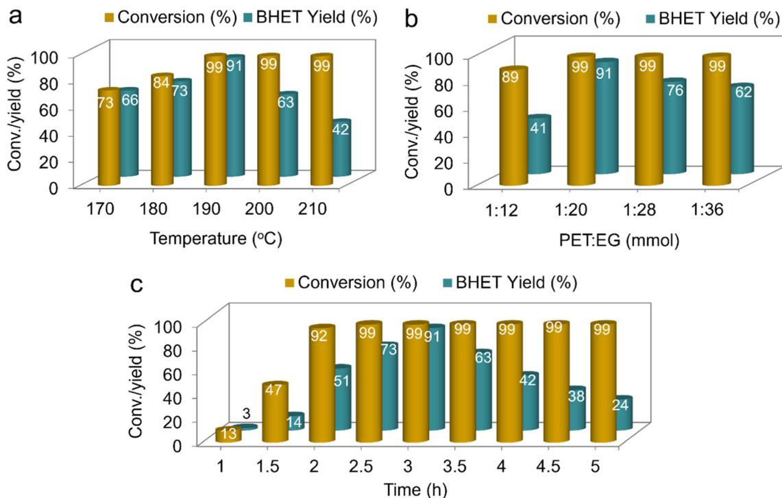
**Fig. 7** Optimization of the reaction conditions for PET glycolysis using the  $\text{MnO}_x/\text{TiO}_2\text{-NR}$  catalyst: (a) temperature, (b) PET/EG molar ratio, and (c) reaction time. Reaction conditions: 1 : 20 molar ratio of PET : EG, 5 wt%  $\text{MnO}_x/\text{TiO}_2\text{-NR}$  catalyst, 190 °C, and 3 h. Error in isolated BHET yield:  $\pm 3\%$ .
