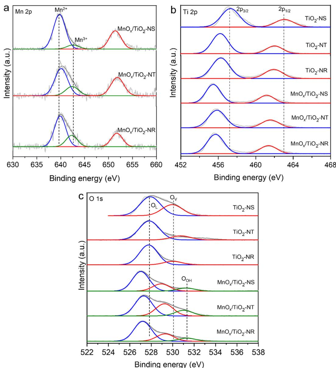
Fig. 5 (a) Mn 2p, (b) Ti 2p, and (c) O 1s XPS spectra of TiO<sub>2</sub> and MnO<sub>x</sub>/TiO<sub>2</sub> catalysts.
