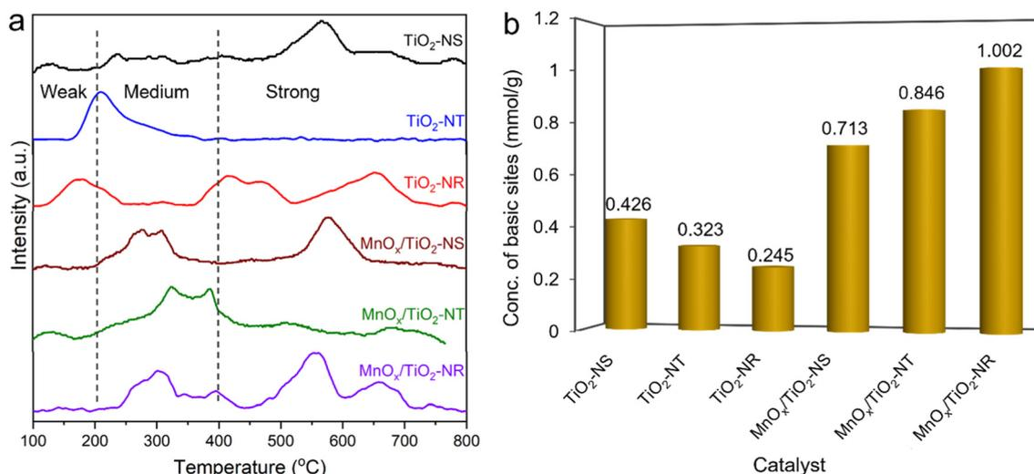
Fig. 6 (a) CO<sub>2</sub>-TPD profiles and (b) basic site concentration of TiO<sub>2</sub> and MnO<sub>x</sub>/TiO<sub>2</sub> catalysts.
