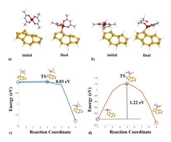
**Fig. 3** (a) Initial and final configurations for reaction C; (b) initial and final configurations for reaction D; (c) detailed pathway progression for reaction C; (d) reaction pathway for reaction D, both highlighting the TS and the respective potential barrier height.
