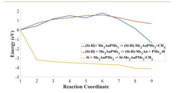
Fig. 6 Au reaction pathways highlighting the absence of a potential barrier for reaction E of Me<sub>3</sub>AuPMe<sub>3</sub> with bare silicon, and the comparable barrier height increase of reactions G and F for the adsorption of Me<sub>3</sub>AuPMe<sub>3</sub> onto the hydrogen passivated substrate. The yellow curve represents reaction E, the red curve represents reaction G, and the blue curve represents reaction F
