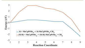
Fig. 2 MeCpPtMe<sub>3</sub> reaction pathways. Reaction A pathway is in blue, reaction B is in red; the difference in barrier height is relevant and suggests deposition selectivity of the process.
