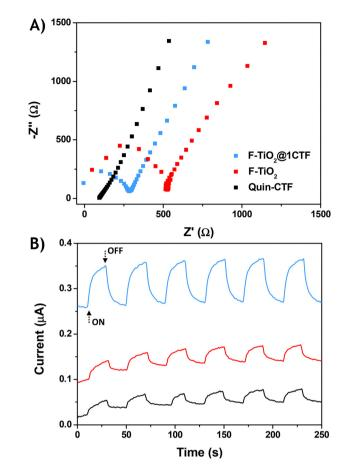
Fig. 6 Electrochemical studies of F-TiO<sub>2</sub>, F-TiO<sub>2</sub>@1CTF and Quin-CTF in Na<sub>2</sub>SO<sub>4</sub> 0.2 M vs. Ag/AgCl (3 M KCl). (A) Nyquist plots obtained without applying bias and (B) photocurrent response at a potential of 0.6 V vs. Ag/AgCl (3 M KCl) under irradiation with UV-vis light.
