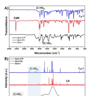
Fig. 1 (A) FT-IR spectra and (B) <sup>13</sup>C-NMR spectra of the organic precursors Quin-I (blue curves), Quin-CN (red curves) and Quin-CTF (black curves), highlighting with colored areas the main signals.
