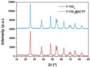
Fig. 3 X-ray diffractograms of F-TiO<sub>2</sub> and F-TiO<sub>2</sub>@2CTF materials.
