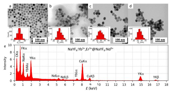
Fig. 1 TEM micrographs of (a) C-UCNPs, (b) CS-UCNPs, (c) CS-UCNP@P(DMA-AEA)-Ale, (d) CS-UCNP@P(DMA-AEA)-Ale-Hyp particles and (e) EDX of CS-UCNPs.
