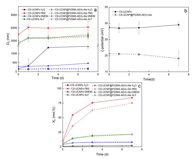
Fig. 3 Time dependence of (a) hydrodynamic diameter  $D_{h_z}$  (b)  $\zeta$ -potential and (c)  $F^-$  ion mole fraction ( $X_F$ ) of CS-UCNPs and CS-UCNPs P(DMA-AEA)-Ale particles in supernatants after incubation of particles in water, PBS (pH = 7.4), DMEM and ALF at 37 °C.
