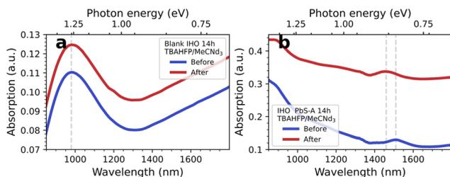
Fig. 3 (a) Blank IHO before and after 14 h in TBAHFPP/MeCN- $d_3$ . (b) PbS-A film on IHO before and after 14 h in TBAHFPP/MeCN- $d_3$ .
