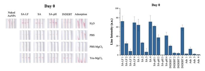
Fig. 6 Lateral flow results of day 0. Left, lateral flow strips. Right, ImageJ quantification. 1 = water, 2 = PBS, 3 = PBS-MgCl<sub>2</sub>, 4 = Tris-MgCl<sub>2</sub>.
