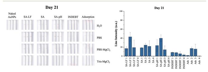
Fig. 7 Lateral flow results of day 21. Left, lateral flow strips. Right, ImageJ quantification. 1 = water, 2 = PBS, 3 = PBS-MgCl<sub>2</sub>, 4 = Tris-MgCl<sub>2</sub>
