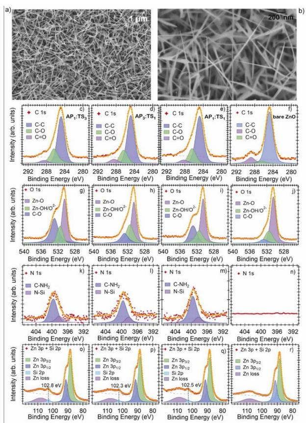
**Fig. 17** (a, b) SEM images of the bare ZnO NWs at different magnifications. XPS spectra of: C 1s (c–f), O 1s (g–j), N 1s (k–n), Zn 3p and Si 2p (o–r). Red markers denote the experimental trace, the orange line is the fit, and the dashed line is the background. The Voigt peaks are included under each spectrum, along with their physical interpretation. ZnO data. Reproduced from ref. 51 with permission from Elsevier, copyright 2023.
