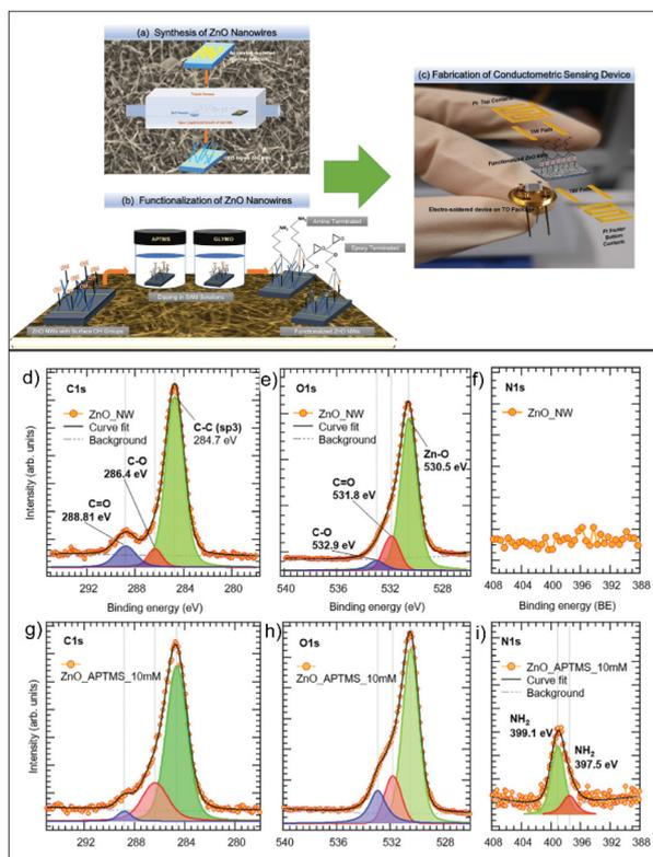
**Fig. 14** (a) Synthesis of ZnO nanowires using the vapor–liquid–solid (VLS) mechanism, (b) surface functionalization of ZnO nanowires with APTMS and GLYMO self-assembled monolayers, and (c) conductometric sensing device. (d–f) XPS spectra for bare ZnO NW (first row), (g–i) APTMS (second row). Reproduced from ref. 46 with permission from Wiley, copyright 2020.
