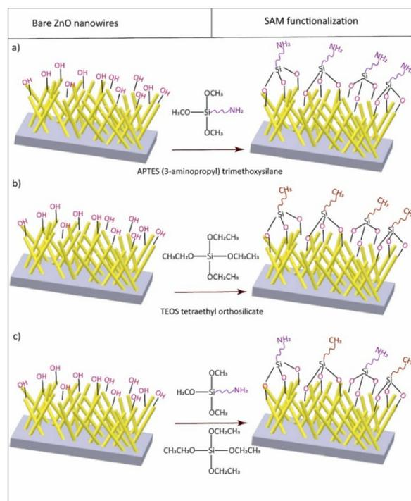
Fig. 3 Functionalization strategy of ZnO nanowires with homogeneous SAMs of APTES (a) and TEOS (b) monolayers, which leads to the formation of amine (-NH<sub>2</sub>) and methyl (-CH<sub>3</sub>) terminated ZnO nanowires, respectively. In panel c, ZnO nanowires were functionalized with a mixture of APTES and TEOS monolayers in a different ratio. Reproduced from ref. 51 with permission from Elsevier B.V., copyright 2023.
