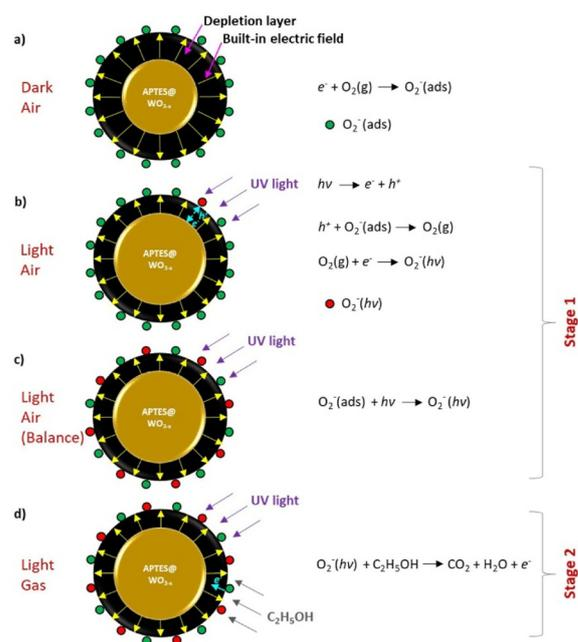
**Fig. 13** Schematic of the gas-sensing mechanism of the UV-LED-activated, APTES-modified WO<sub>3-x</sub> sensor under different conditions: (a) exposed to dry air in the dark, (b) exposed to dry air under UV light, (c) exposed to dry air under UV light after achieving oxygen adsorption/desorption balance, (d) exposed to ethanol under UV light. Reproduced from ref. 60 with permission from Elsevier, copyright 2021.
