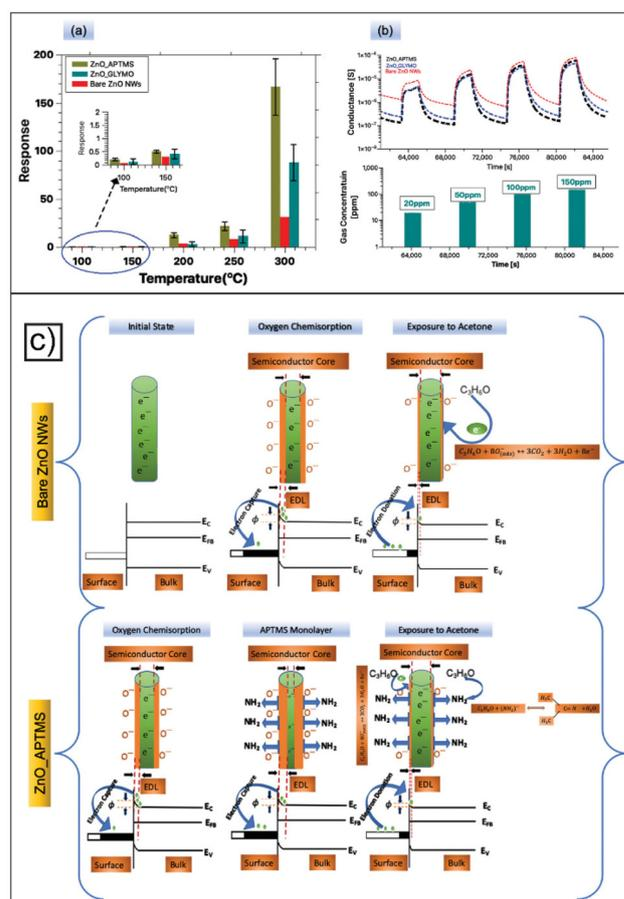
**Fig. 15** (a) Response *versus* temperature plot. (b) Dynamic response (at 300 °C) of bare and SAM ( $10 \times 10^{-3}$  m APTMS and GLYMO) functionalized ZnO nanowires recorded in dry air. (c) Gas-sensing mechanism of bare and SAM ( $10 \times 10^{-3}$  m APTMS) functionalized ZnO NWs for acetone detection. Reproduced from ref. 46 with permission from Wiley, copyright 2020.
