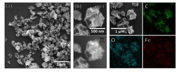
Fig. 1 SEM micrographs of the CG/Fe nanocomposite: secondary electrons (a), (b-i), and backscattered electrons (b-ii); (c) EDS mapping of the CG/ Fe composite with the presence of carbon (C), oxygen (O), and (Fe) iron species.
