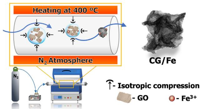
Scheme 1 Synthetic scheme of the CG/Fe composite.
