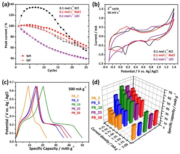
Fig. 5 Stability of the peak current as a function of CV over 25 CV cycles (a) and voltammetric profiles in 0.1 mol L<sup>-1</sup> KCl (black line), 0.1 mol L<sup>-1</sup> NaCl (red line), and 0.1 mol L<sup>-1</sup> LiCl (purple line) (b) – measurements were taken at 50 mV s<sup>-1</sup>; galvanostatic charge–discharge curves at 500 mA g<sup>-1</sup> in 0.1 mol  $L^{-1}$  KCl (c); and specific capacities of the electrodes at different current densities in 0.1 mol  $L^{-1}$  KCl (d).
