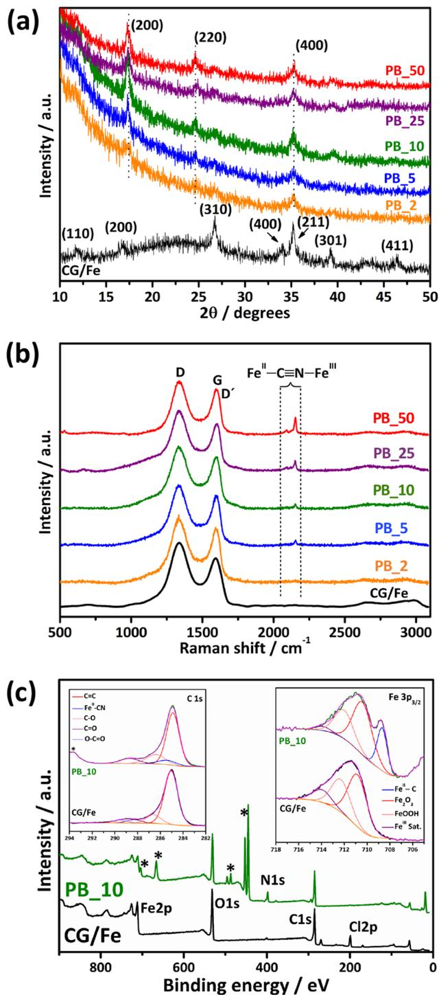
Fig. 3 X-ray diffractograms (a) and Raman spectra ( $\lambda = 633 \text{ nm}$ ) (b) of the CG/Fe (black line), PB\_2 (orange line), PB\_5 (blue line), PB\_10 (green line), PB\_25 (purple line), and PB\_50 (red line) samples. XPS spectra of the CG/Fe and PB\_10 samples (c).
