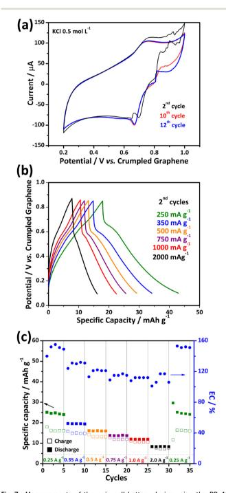
Fig. 7 Measurements of the coin cell battery device using the PB\_10 sample as a cathode and bare\_CG as an anode. (a) Cyclic voltammetry profiles at 50 mV s<sup>-1</sup>, (b) charge/discharge profiles, and (c) rate handling performance.
