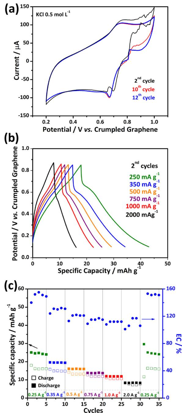
Fig. 7 Measurements of the coin cell battery device using the PB<sub>10</sub> sample as a cathode and bare<sub>CG</sub> as an anode. (a) Cyclic voltammetry profiles at 50 mV s<sup>-1</sup>, (b) charge/discharge profiles, and (c) rate handling performance.
