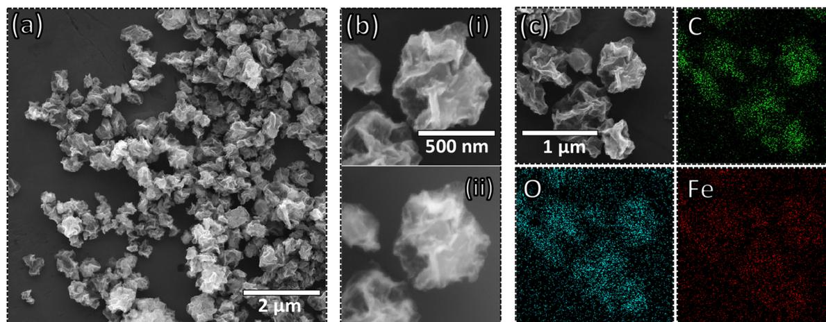
**Fig. 1** SEM micrographs of the CG/Fe nanocomposite: secondary electrons (a), (b-i), and backscattered electrons (b-ii); (c) EDS mapping of the CG/Fe composite with the presence of carbon (C), oxygen (O), and (Fe) iron species.
