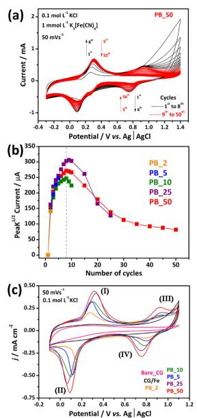
Fig. 2 Electrodeposition of PB nanocubes performed in fifty cycles at a scan rate of 50 mV  $\rm s^{-1}$  in 0.1 mol  $\rm L^{-1}$  KCl electrolyte and 0.1 mmol  $\rm L^{-1}$ K<sub>3</sub>[Fe(CN)<sub>6</sub>] for the PB\_50 sample (a). Cathodic peak (between 0.90 and 0.55 V) current intensity as a function of the voltammetric cycles (b). Cyclic voltammograms for the modified electrodes: CG/Fe (black line) and pure CG (pink line) films before electrodeposition (c).
