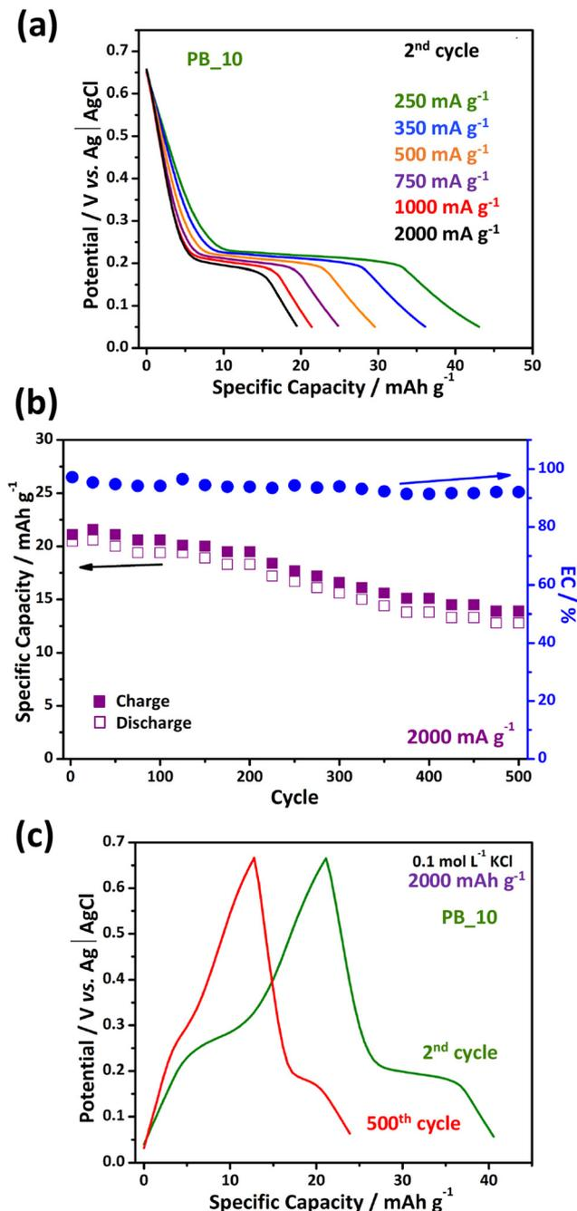
Fig. 6 Measurements of the PB<sub>10</sub> sample. (a) Discharge profiles at different rate, (b) stability test at 2000 mA g<sup>-1</sup>, and (c) charge/discharge stability test profiles.
