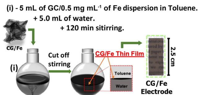
Scheme 2 Experimental step to prepare CG/Fe films at the liquid-liquid interface.
