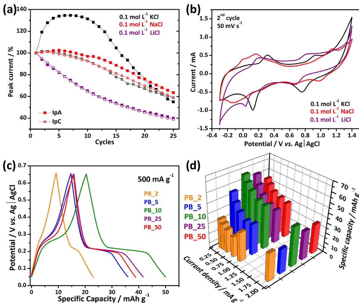
Fig. 5 Stability of the peak current as a function of CV over 25 CV cycles (a) and voltammetric profiles in 0.1 mol L<sup>-1</sup> KCl (black line), 0.1 mol L<sup>-1</sup> NaCl (red line), and 0.1 mol L<sup>-1</sup> LiCl (purple line) (b) – measurements were taken at 50 mV s<sup>-1</sup>; galvanostatic charge–discharge curves at 500 mA g<sup>-1</sup> in 0.1 mol L<sup>-1</sup> KCl (c); and specific capacities of the electrodes at different current densities in 0.1 mol L<sup>-1</sup> KCl (d).
