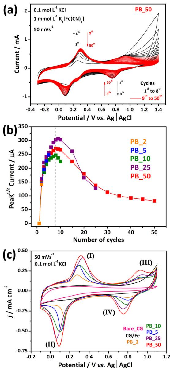
**Fig. 2** Electrodeposition of PB nanocubes performed in fifty cycles at a scan rate of  $50 \text{ mV s}^{-1}$  in  $0.1 \text{ mol L}^{-1} \text{ KCl}$  electrolyte and  $0.1 \text{ mmol L}^{-1} \text{ K}_3[\text{Fe}(\text{CN})_6]$  for the PB\_50 sample (a). Cathodic peak (between 0.90 and 0.55 V) current intensity as a function of the voltammetric cycles (b). Cyclic voltammograms for the modified electrodes: CG/Fe (black line) and pure CG (pink line) films before electrodeposition (c).
