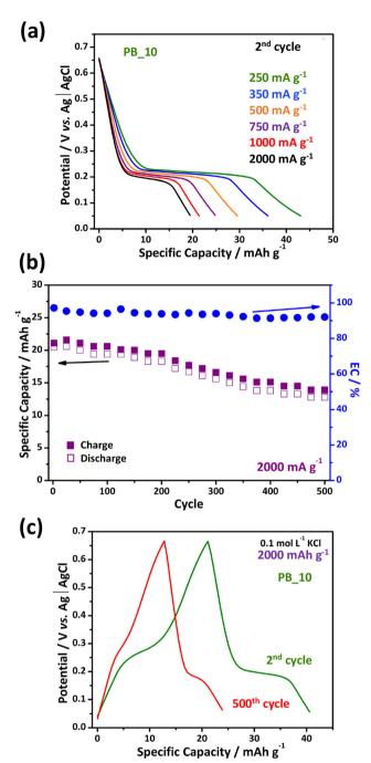
Fig. 6 Measurements of the PB\_10 sample. (a) Discharge profiles at different rate, (b) stability test at 2000 mA g<sup>-1</sup>, and (c) charge/discharge stability test profiles.
