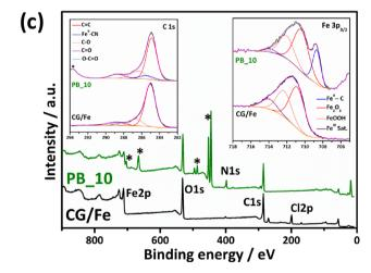
Fig. 3 X-ray diffractograms (a) and Raman spectra ( $\lambda$  = 633 nm) (b) of the CG/Fe (black line), PB\_2 (orange line), PB\_5 (blue line), PB\_10 (green line), PB\_25 (purple line), and PB\_50 (red line) samples. XPS spectra of the CG/Fe and PB\_10 samples (c).
