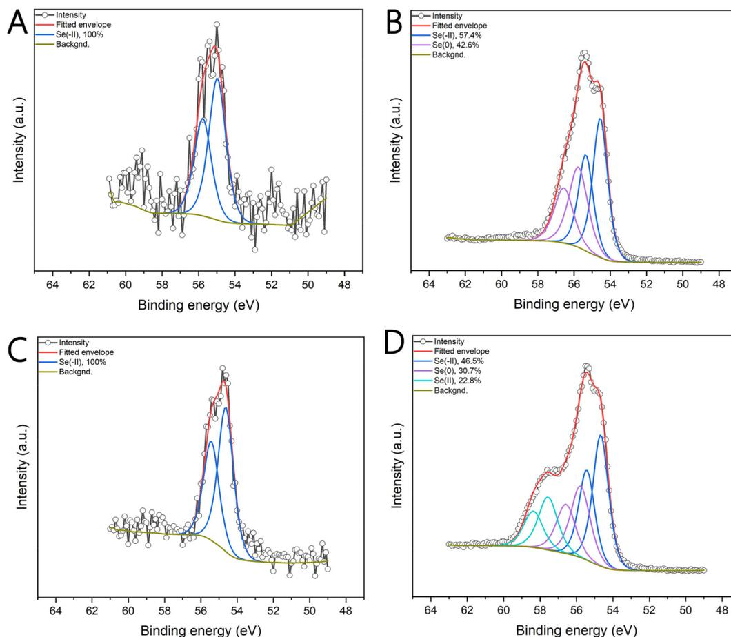
**Fig. 5** The X-ray photoelectron spectra (XPS) of selenium (Se 3d) for (A) destabilized SeNPs reduced by  $\text{NaBH}_4$ , (B) SeNPs in a stable state reduced by  $\text{NaBH}_4$ , (C) gray destabilized SeNPs reduced by ascorbic acid, and (D) orange stable SeNPs reduced by ascorbic acid.
