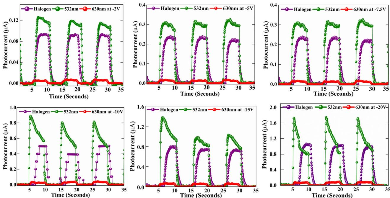
Fig. 5 Photocurrent analysis in response to illumination with a halogen lamp, 532 nm laser, and 630 nm laser fixed at  $-2$  V,  $-5$  V,  $-7.5$  V,  $-10$  V,  $-15$  V, and  $-20$  V, respectively.
