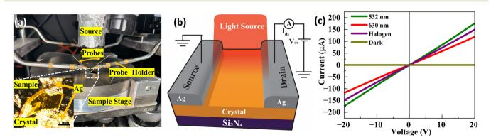
Fig. 2 (a) Experimental setup: MPS150 Cascade Microtech EPS150TRIAX probe station. Inset shows the optical image of the crystal. (b) Schematics of the photocurrent measurement. (c) I-V curves of Form A1 crystal under 532 nm, 630 nm, and halogen illumination and in the dark.
