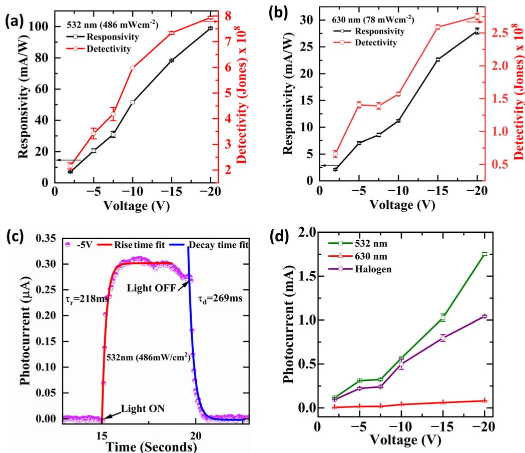
**Fig. 6** Responsivity and detectivity of the device under (a) 532 nm and (b) 630 nm illumination. (c) Decay and rise times of photocurrent. (d) Photocurrent vs. voltage response under 532 nm, 630 nm and halogen illumination.
