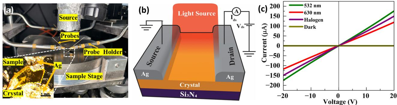
Fig. 2 (a) Experimental setup: MPS150 Cascade Microtech EPS150TRIAx probe station. Inset shows the optical image of the crystal. (b) Schematics of the photocurrent measurement. (c)  $I$ - $V$  curves of Form A1 crystal under 532 nm, 630 nm, and halogen illumination and in the dark.
