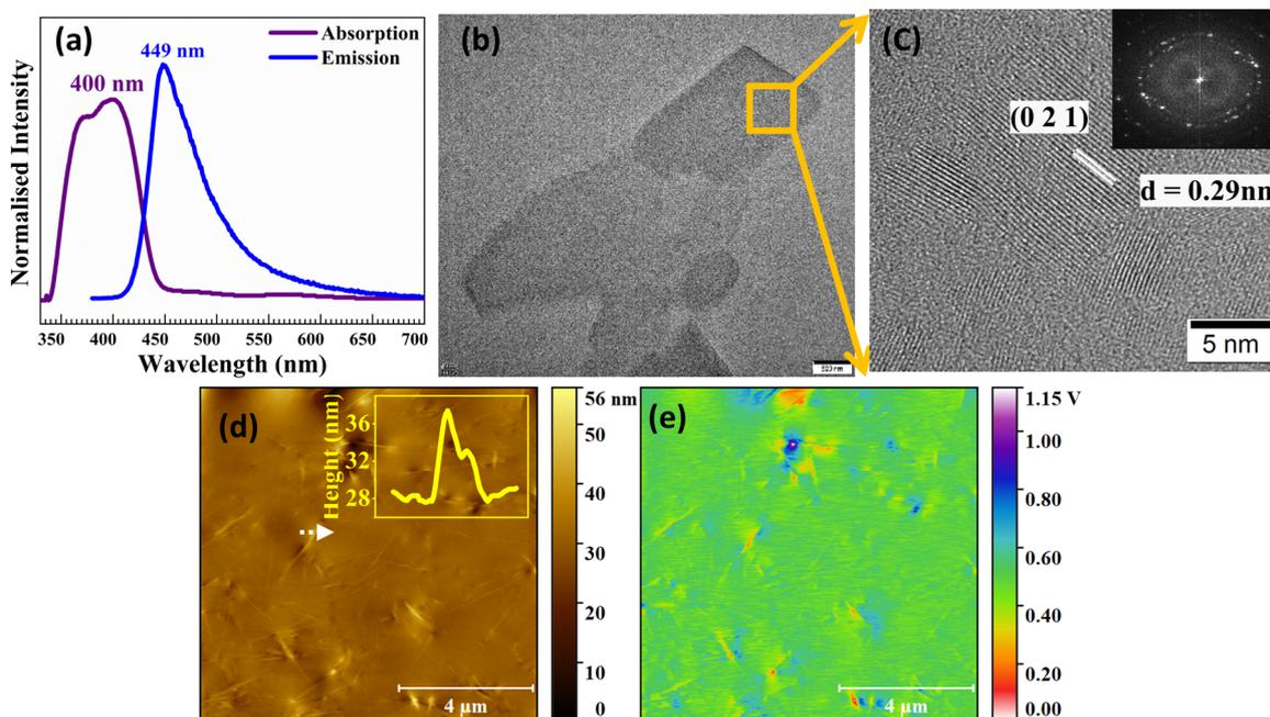
**Fig. 3** (a) The Form A1 absorption and photoemission spectra, (b and c) HRTEM image of the crystal (inset shows the SAED pattern), (d) AFM micrograph of the crystal with the inset illustrating the height profile indicated by the white dashed line, and (e) surface potential map obtained by KPFM.
