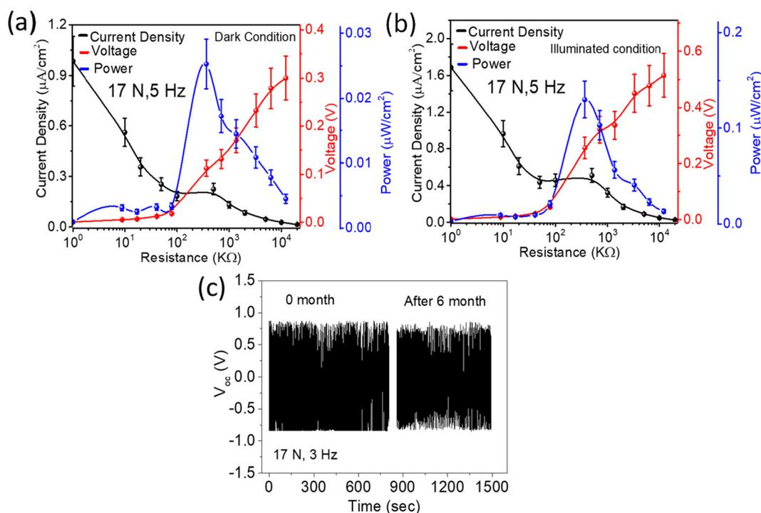
**Fig. 6** Variation of  $J$ ,  $V$ , and  $P$  output with load resistance in (a) dark conditions, (b) light-illuminated conditions. (c) Fatigue test over 20 000 cycles and after 6 months at 17 N and 5 Hz.
