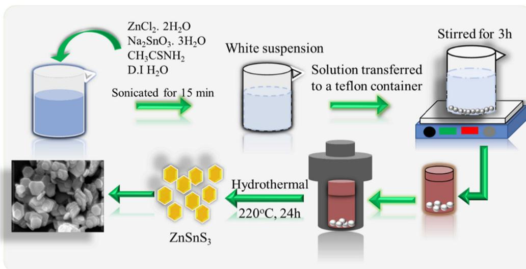
**Scheme 1** Synthesis process scheme for LN-ZnSnS<sub>3</sub> nanocrystals.
