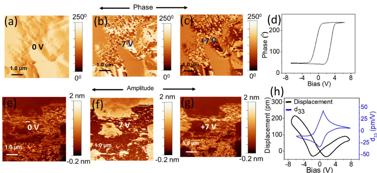
Fig. 3 PFM (a)–(c) phase images with a change of bias voltage  $\pm 7$  V of the LN-ZTS NC film. (d) Plot of the phase change of the LN-ZTS NC film. (e)–(g) Amplitude images with the same change in bias voltage. (h) Butterfly loop and  $d_{33}$  plot.
