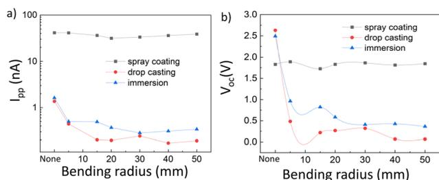
**Fig. 5** Summary of measurements after bending tests with varying bending radii, ranging from no bending to 50 mm, for the samples produced by the three different deposition methods. Panel (a) shows the peak-to-peak short-circuit current ( $I_{pp}$ ) and panel (b) shows the open-circuit voltage. The counter triboelectric layer is PVC for drop casting and immersion and nylon for spray coating.
