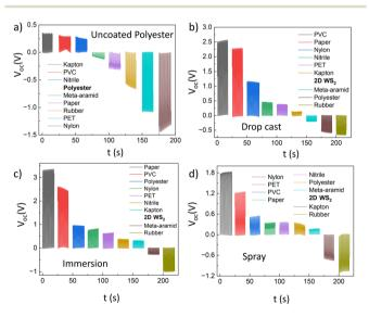
**Fig. 3** Triboelectric series based on open-circuit voltage measurements over time for different triboelectric layers of TENGs tested with (a) uncoated polyester, (b) polyester coated with 2D WS<sub>2</sub> via drop casting, (c) polyester coated with 2D WS<sub>2</sub> via immersion, and (d) polyester coated with 2D WS<sub>2</sub> via spray.
