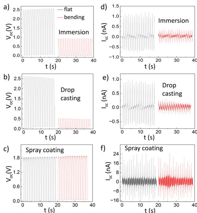
**Fig. 4** Open-circuit voltage and short-circuit current of TENG devices in the flat position and after bending 5 mm with the 2D WS<sub>2</sub> device prepared by immersion (a and d), drop casting (b and e), and spray coating (c and f). The counter triboelectric layer is PVC for drop casting and immersion and nylon for spray coating.
