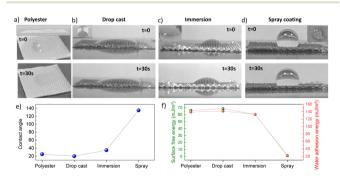
**Fig. 6** Photographs of the water contact angle for polyester (a) and polyester coated with 2D  $WS_2$  by drop casting (b), immersion (c), and spray coating (d). The wettability measurement was carried out using a goniometer and the contact angle (e) was analysed using an online screen protractor. (f) Surface free energies and water adhesion energies for the different samples.
