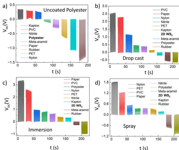
**Fig. 3** Triboelectric series based on open-circuit voltage measurements over time for different triboelectric layers of TEMGs tested with (a) uncoated polyester, (b) polyester coated with 2D  $\text{WS}_2$  via drop casting, (c) polyester coated with 2D  $\text{WS}_2$  via immersion, and (d) polyester coated with 2D  $\text{WS}_2$  via spray.
