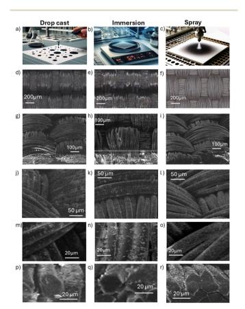
higher magnification imaging for precise thickness measurement was hindered by charging effects due to the non-conductive fabric substrate.
