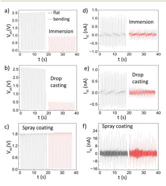
**Fig. 4** Open-circuit voltage and short-circuit current of TENG devices in the flat position and after bending 5 mm with the 2D  $WS_2$  device prepared by immersion (a and d), drop casting (b and e), and spray coating (c and f). The counter triboelectric layer is PVC for drop casting and immersion and nylon for spray coating.
