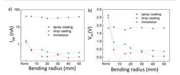
**Fig. 5** Summary of measurements after bending tests with varying bending radii, ranging from no bending to 50 mm, for the samples produced by the three different deposition methods. Panel (a) shows the peak-to-peak short-circuit current ( $l_{pp}$ ) and panel (b) shows the opencircuit voltage. The counter triboelectric layer is PVC for drop casting and immersion and nylon for spray coating.
