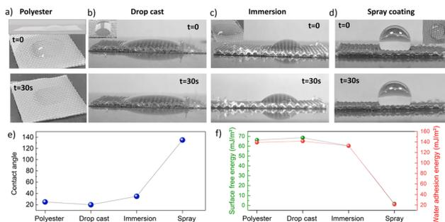
**Fig. 6** Photographs of the water contact angle for polyester (a) and polyester coated with 2D WS<sub>2</sub> by drop casting (b), immersion (c), and spray coating (d). The wettability measurement was carried out using a goniometer and the contact angle (e) was analysed using an online screen protractor. (f) Surface free energies and water adhesion energies for the different samples.
