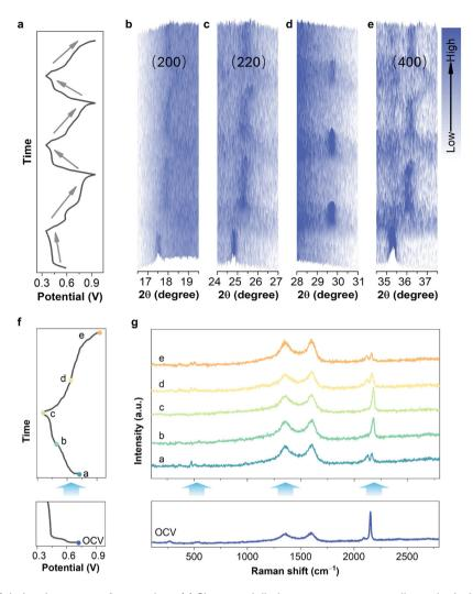
Fig. 4 Evolution of FeHCF during the storage of copper ions. (a) Charge and discharge curves corresponding to *in situ* XRD of the FeHCF electrode. (b–e) The *in situ* XRD curve of FeHCF corresponding to (a). (f) Charge and discharge curves and (g) Raman spectra of FeHCF at the corresponding potentials in (f).
