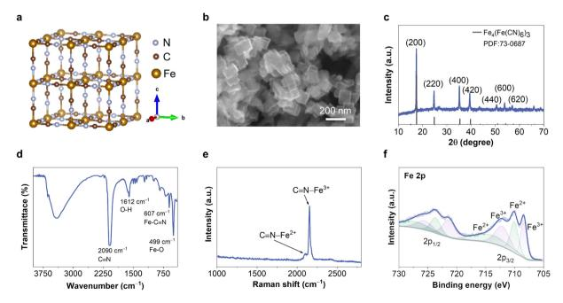
Fig. 1 Morphology, structure and chemical composition of FeHCF. (a) The cubic crystal structure and (b) scanning electron microscopy (SEM) image of FeHCF. (c) XRD patterns, (d) FTIR spectroscopy and (e) Raman spectra of FeHCF. (f) XPS spectra of Fe 2p for FeHCF.
