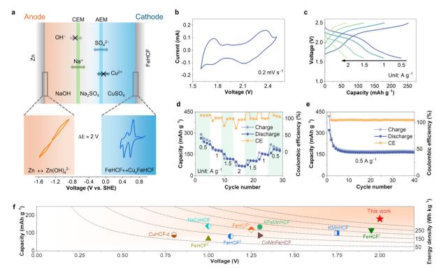
Fig. 6 Performance of the Zn//FeHCF decoupled battery. (a) Structure and mechanism diagram of the Zn//FeHCF decoupled battery. (b) CV curves recorded at 0.2 mV s<sup>-1</sup>. (c) GCD curves at different current densities. (d) Rate performance of the Zn//FeHCF decoupled battery. (e) Electrochemical cycling stability at a fixed rate of 0.5 A g<sup>-1</sup>. (f) Comparison of the Zn//FeHCF decoupled battery with recently reported batteries using PBAs as
