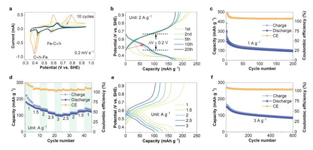
Fig. 2 Electrochemical copper-ion storage performance of FeHCF. (a) In situ CV curves recorded at 0.2 mV s<sup>-1</sup>. (b) Change of the GCD curves of FeHCF. (c) Long-term cycling of the FeHCF electrode (FeHCF: super P: PVDF = 7:2:1) in 1 M CuSO<sub>4</sub> solution at a fixed rate of 1 A g<sup>-1</sup>. (d) Rate performance and (e) GCD curves of FeHCF at different current densities. (f) Long-term cycling of FeHCF at a fixed rate of 3 A  $\rm g^{-1}$ .
