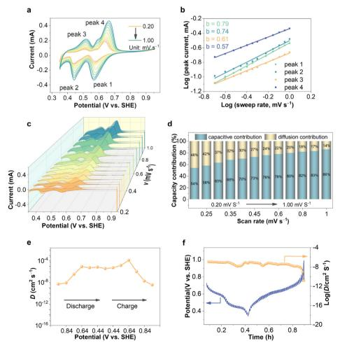
Fig. 3 (a) CV curves of FeHCF at various scan rates. (b) Plots of log(i) versus log(v) of FeHCF. (c and d) The pseudocapacitive and diffusion-controlled charge storage contributions at different scan rates of FeHCF. (e) Diffusion coefficient as a function of potential derived from the impedance spectra. (f) Diffusion coefficient of copper-ion of FeHCF measured by the GITT.
