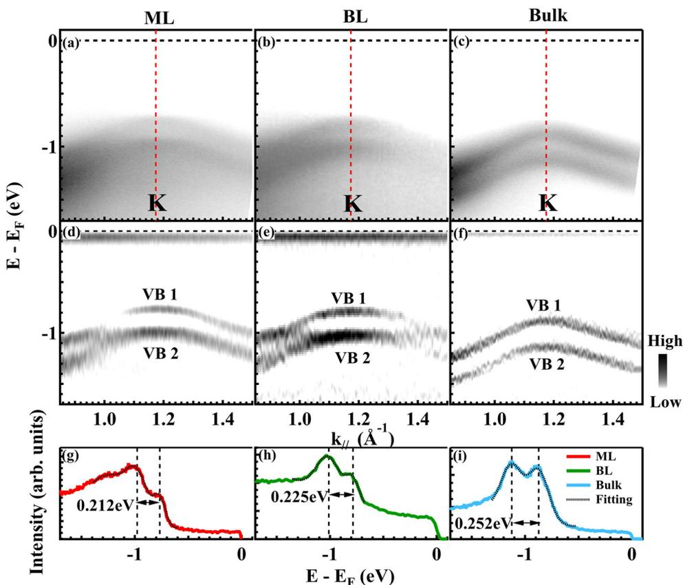
Fig. 4 Layer dependent band splitting at K. (a-c) ARPES maps showing the valence band splitting around K along the  $\Gamma$ -K-M direction for ML, BL and bulk MoTe<sub>2</sub>, respectively. (d-f) Second derivative spectra of (a-c) along the energy axis, respectively. (g-i) EDCs at K from (a-c), shown as red (ML), green (BL) and blue (bulk) curves, respectively. The black dotted curves are the corresponding Gaussian fitting results, with peak positions indicated by black dashed lines.
