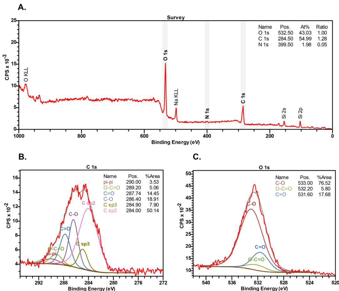
**Fig. 3** XPS survey and high-resolution spectra of AP-LAV-CDs. (A) Survey spectrum annotated with predominant peaks, including substrate-derived Si peaks. Binding energy (BE), atomic percentages, and ratios (relative to C) of shaded peaks are provided. High-resolution core-level spectra of (B) C 1s and (C) O 1s are deconvoluted, with distinct bonding environments labelled.
