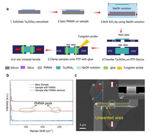
Fig. 6 A schematic showing the typical transfer process for 2D materials samples onto MEMS chips, composed of three steps. (a) The polymer-assisted transfer process onto MEMS chips.<sup>28</sup> (b) Removal of the polymer after transfer, confirmed by Raman spectroscopy.<sup>28</sup> (c) The clamping and shaping of sample under FIB.<sup>28</sup>
