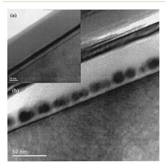
Fig. 2 (a) Cross-section TEM micrograph of the Si<sub>0.54</sub>Ge<sub>0.46</sub> film that has been wet oxidized at 600 °C for 60 min. (b) Cross-section TEM micrograph of the Ge nanodots formed by annealing the structure shown in (a) in N<sub>2</sub> for 300 s at 1000 °C. Reproduced with permission from ref. 74, Copyright 2004, AIP Publishing.
