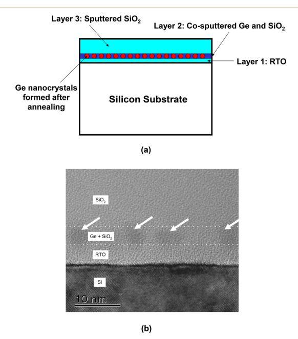
Fig. 1 (a) Schematic diagram of the tri-layer insulator gate stack structure. (b) TEM cross-section showing the formation of germanium nanocrystals (indicated by white arrows) in a 3 nm thick middle layer (bound by dotted white lines) of the tri-layer insulator gate stack structure. (b) Reproduced with permission from ref. 70, Copyright 2002, AIP Publishing.
