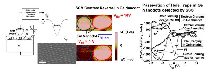
Fig. 9 Scanning capacitance spectroscopy/microscopy (SCS/SCM) of Ge nanodots before and after forming gas annealing at 450 °C showing electron and hole charging in Ge nanodots. Reproduced with permission from ref. 75, Copyright 2008, AIP Publishing.
