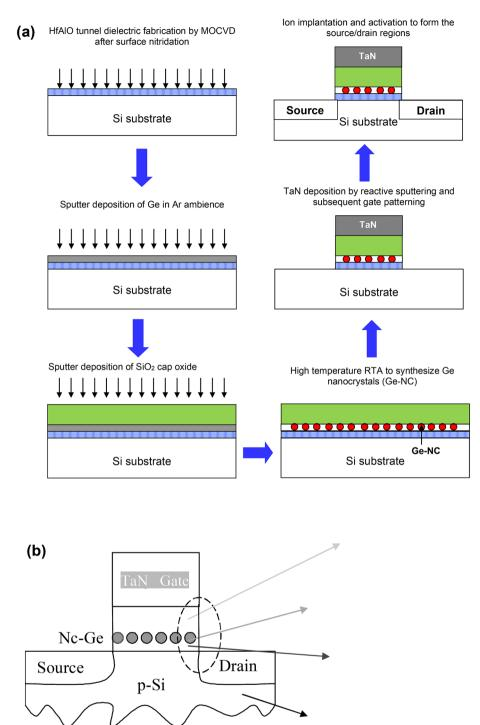
Fig. 3 (a) Schematic diagram of the fabrication process flow of the Ge nanocrystal memory transistor. (b) Schematic and TEM cross-section of the Ge nanocrystal memory transistor showing the Ge nanocrystals formed in the middle layer of the tri-layer gate structure. (a) Reproduced with permission from ref. 73, Copyright 2023, American Chemical Society.
