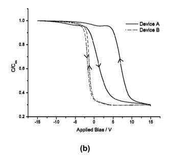
Fig. 4 (a) TEM cross-section showing the formation of germanium nanocrystals in a 20 nm thick middle layer (bound by dotted white lines) of the tri-layer insulator gate stack structure. (b) Anti-clockwise hysteresis in the high frequency *C–V* characteristics of device A (with Ge nanocrystals) indicating the charge storage or memory effect as compared to the negligible hysteresis in control device B (without Ge nanocrystals). Adapted with permission from ref. 69, Copyright 2002, AIP Publishing.
