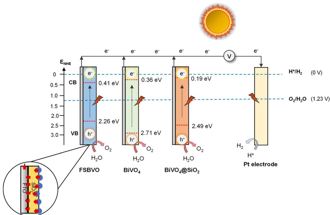
Fig. 9 Proposed mechanism of PEC water splitting over  $\text{BiVO}_4$ -based photoanodes.
