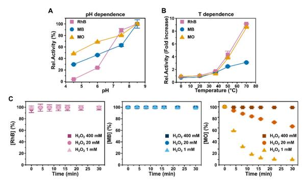
Fig. 2 Effect of pH and temperature on AuNZ performance and comparison with natural HRP enzyme. Degradation of the three dyes by AuNZs as a function of (A) pH and (B) temperature. Data were normalized to the maximum activity obtained with each dye. (C) Natural horseradish peroxidase (20 ppm) shows no activity with RhB (10  $\mu$ M) and MB (14  $\mu$ M), while it can oxidize MO (40  $\mu$ M), when used with low H<sub>2</sub>O<sub>2</sub> concentrations.
