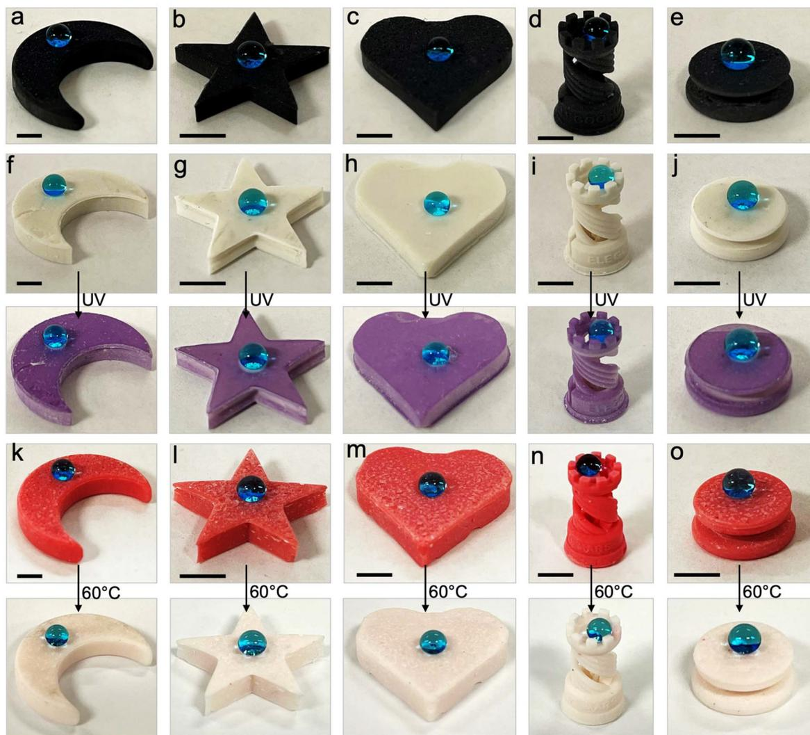
**Fig. 5** 3D printed multifunctional objects. Water droplets (blue) beading up on 3D printed objects of different geometries. (a–e) Magnetic superhydrophobic objects, (f–j) photochromic superhydrophobic objects, before UV exposure (white) and after UV exposure (violet), and (k–o) thermochromic superhydrophobic objects, at 25 °C (red) and at 80 °C (white). Scale bars represent 5 mm.
