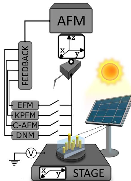
**Fig. 1** Schematic of the AFM with its calibrated  $x$ ,  $y$ ,  $z$  scanner head and its  $x$ ,  $y$  moving sample stage, as a multi-metrological platform with both tip-scan and sample-scan configurations as well as many modes for nanoelectrical and mechanical characterization.
