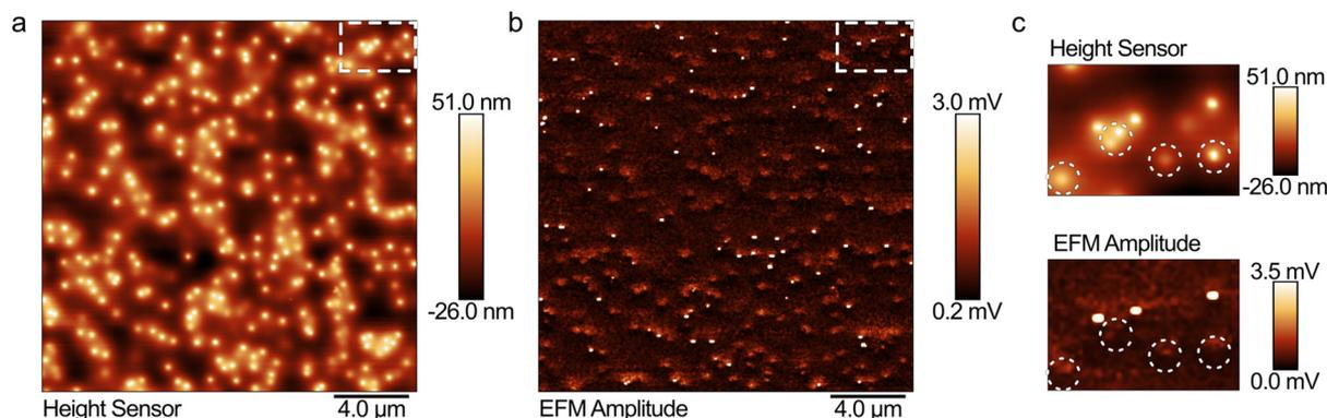
**Fig. 5** EFM measurements of non-passivated GaAs nanowires embedded in a BCB polymer matrix, (a) showing the sample's topography and (b) the variations in the EFM amplitude of the electrostatically driven oscillating cantilever. The difference in individual NW contributions to surface charge is highlighted in (c).
