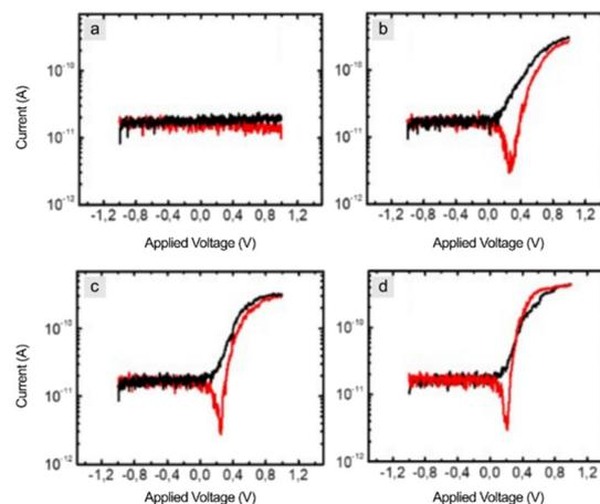
**Fig. 9** Current versus voltage ( $I$ - $V$ ) curves measured by contacting individual nanowires across the array. (a) Example of a non-responsive nanowire. (b-d) Electrically responsive nanowires showing diode-like and pseudo-photovoltaic behaviours. Black lines correspond to the forward sweep of the bias (increasing voltage) and red lines correspond to the reverse sweep.
