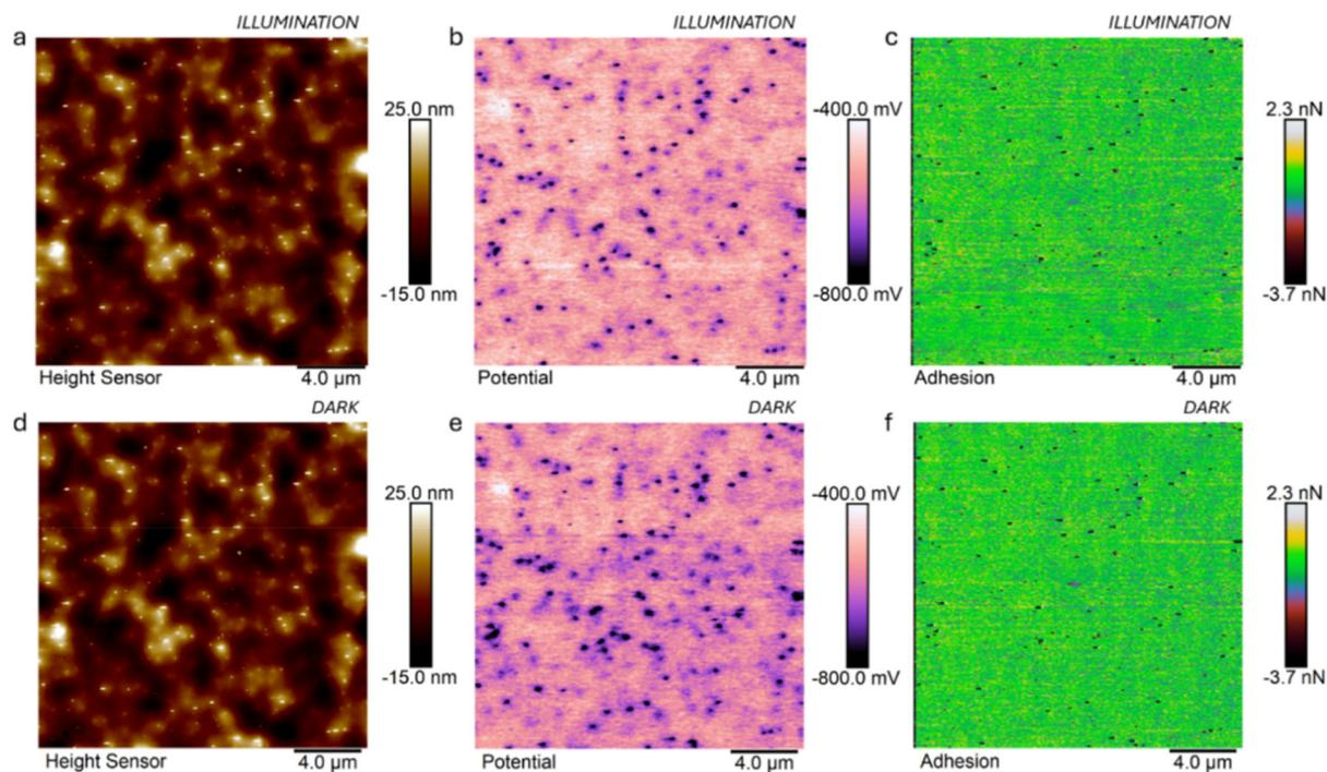
**Fig. 6** (a–c) Topography, surface potential, and adhesion maps, respectively, measured in PF KPFM under illumination conditions on the sample of non-passivated vertical nanowire array (non-passivated). (d–f) Same measurements performed under dark conditions.
