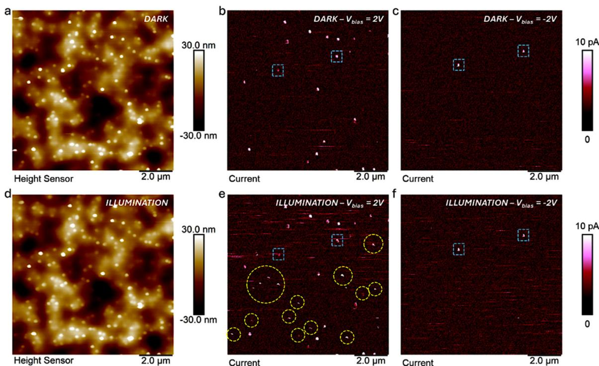
**Fig. 8** C-AFM measurements of non-passivated GaAs NWs under dark and under illumination conditions showing (a and d) the surface topography maps and current maps measured with an applied  $V_{\text{bias}} = 2\text{ V}$  (b and e) and  $V_{\text{bias}} = -2\text{ V}$  (c and f).
