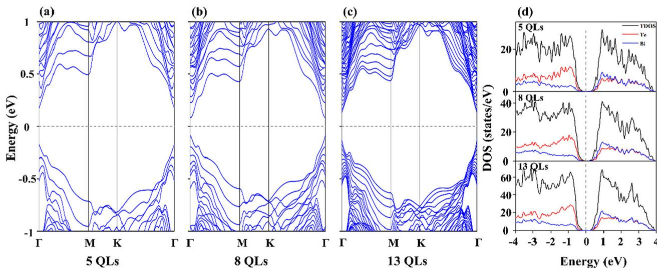
**Fig. 4** The band structures of Bi<sub>2</sub>Te<sub>3</sub> of (a) 5 QLs, (b) 8 QLs and (c) 13 QLs. (d) Density of states of 5 QL, 8 QL and 13 QL Bi<sub>2</sub>Te<sub>3</sub> under the PBE functional.
