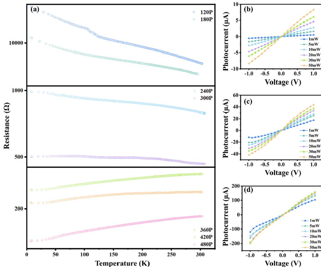
**Fig. 2** (a) Temperature dependence of resistance of  $\text{Bi}_2\text{Te}_3$  thin films with different pulse numbers. The relationship between photocurrent and incident light power for  $\text{Bi}_2\text{Te}_3$  thin films with varying pulse numbers. (b) 120 P, (c) 300 P, and (d) 480 P.
