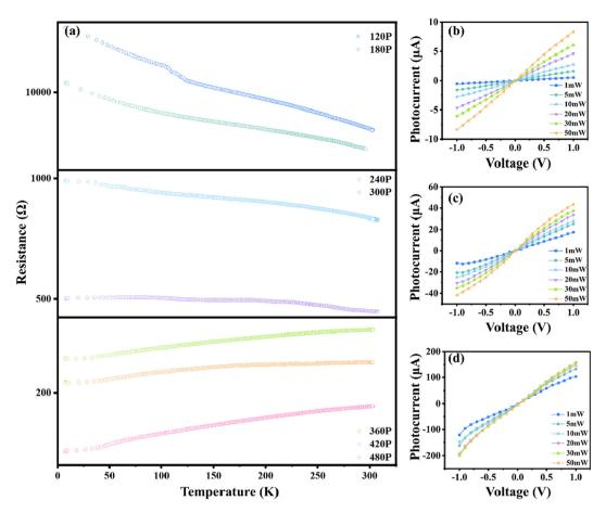
Fig. 2 (a) Temperature dependence of resistance of  $Bi_2Te_3$  thin films with different pulse numbers. The relationship between photocurrent and incident light power for  $Bi_2Te_3$  thin films with varying pulse numbers. (b) 120 P, (c) 300 P, and (d) 480 P.
