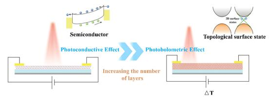
Fig. 5 Photoresponse mechanism diagram of few-layer and multi-layer Bi<sub>2</sub>Te<sub>3</sub> films.
