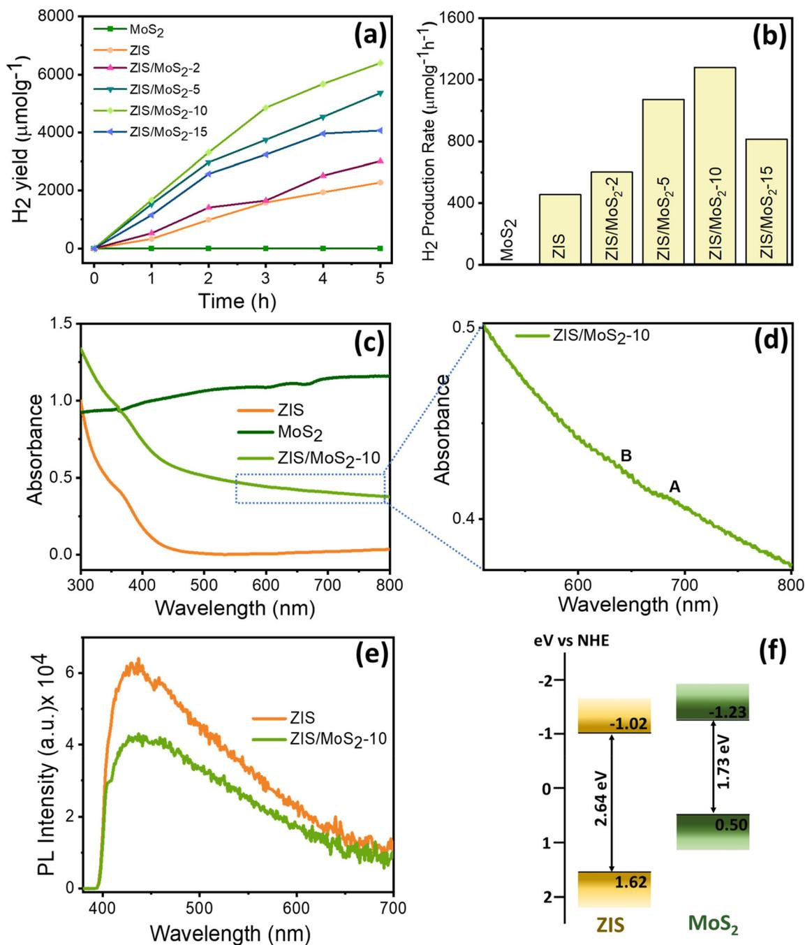
**Fig. 2** H<sub>2</sub> production (a) yields and (b) rates of ZIS, MoS<sub>2</sub>, ZIS/MoS<sub>2</sub>-2, ZIS/MoS<sub>2</sub>-5, ZIS/MoS<sub>2</sub>-10 and ZIS/MoS<sub>2</sub>-15 heterostructures. (c) Steady-state absorption spectra of ZIS, MoS<sub>2</sub>, and ZIS/MoS<sub>2</sub>-10. (d) Enlarged view for ZIS/MoS<sub>2</sub>-10. (e) Photoluminescence spectra of ZIS and ZIS/MoS<sub>2</sub>-10 after photoexcitation at 350 nm. (f) Band position estimation for ZIS and MoS<sub>2</sub>.
