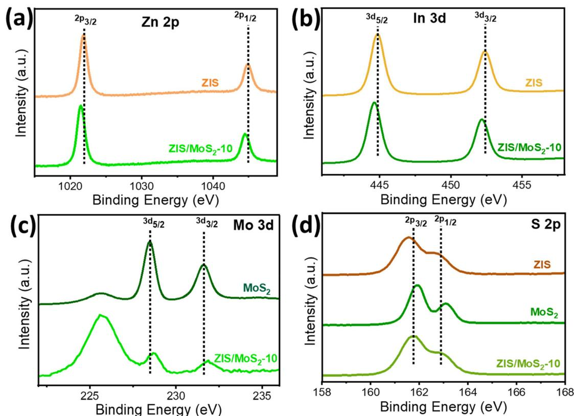
Fig. 3 High-resolution XPS spectra of (a) Zn 2p and (b) In 3d for ZIS and ZIS/MoS<sub>2</sub>-10 and (c) Mo 3d for MoS<sub>2</sub> and ZIS/MoS<sub>2</sub>-10. (d) S 2p for ZIS, MoS<sub>2</sub> and ZIS/MoS<sub>2</sub>-10.
