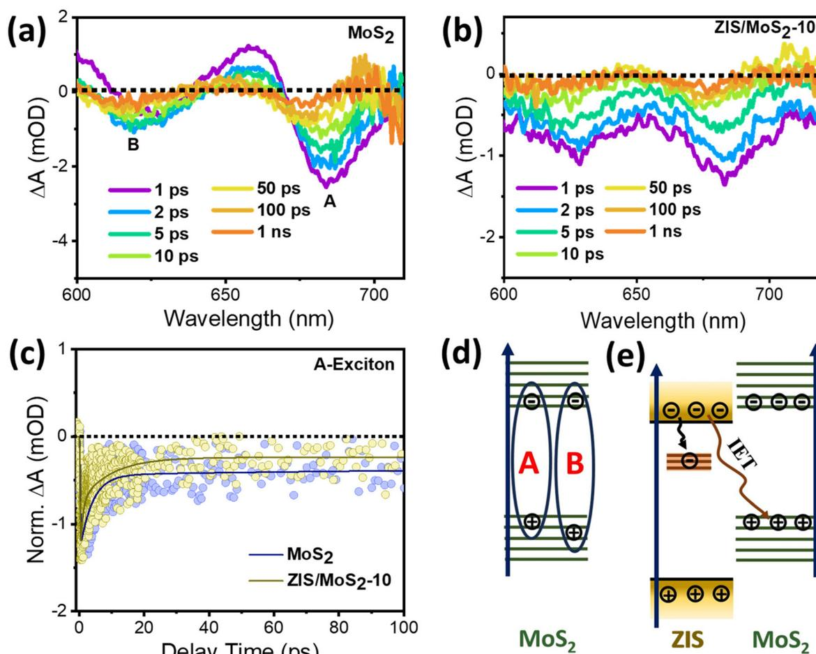
Fig. 5 TA spectra of (a) MoS<sub>2</sub> and (b) the ZIS/MoS<sub>2</sub>-10 heterostructure after photoexcitation at 370 nm. (c) Comparative TA kinetics of MoS<sub>2</sub> and ZIS/MoS<sub>2</sub>-10, monitored at the A excitonic position (687 nm). Ultrafast photophysical processes like the formation of A and B excitons and IET in (d) MoS<sub>2</sub> and (e) the ZIS/MoS<sub>2</sub> heterostructure.
