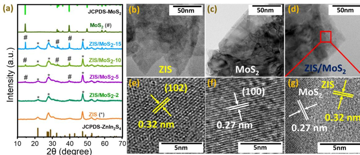
**Fig. 1** (a) XRD pattern of the as-synthesised ZIS, MoS<sub>2</sub>, ZIS/MoS<sub>2</sub>-2, ZIS/MoS<sub>2</sub>-5, ZIS/MoS<sub>2</sub>-10 and ZIS/MoS<sub>2</sub>-15 heterostructures. TEM and HRTEM images of the as-synthesized (b and e) ZIS, (c and f) MoS<sub>2</sub>, (d and g) the ZIS/MoS<sub>2</sub>-10 heterostructure.
