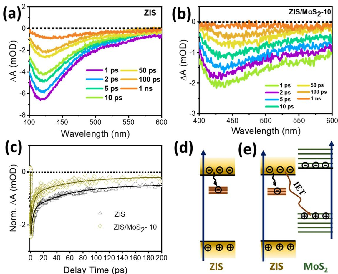
**Fig. 4** TA spectra of (a) ZIS nanosheets and (b) the ZIS/MoS<sub>2</sub>-10 heterostructure after photoexcitation at 370 nm. (c) Comparative TA kinetics of ZIS and ZIS/MoS<sub>2</sub>-10, monitored at 420 nm. Ultrafast photophysical processes, such as electron trapping and interfacial electron transfer (IET) processes in (d) bare ZIS and (e) the ZIS/MoS<sub>2</sub> heterostructure.
