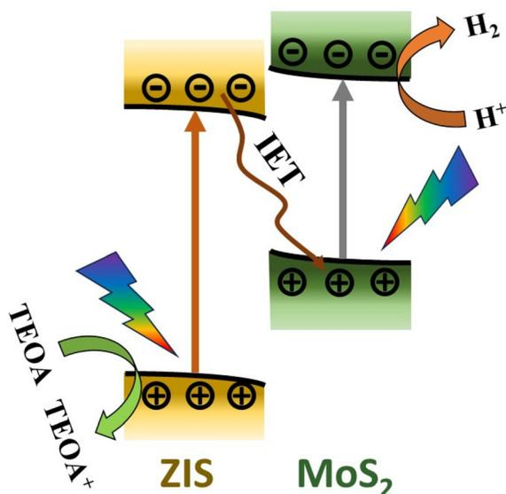
Fig. 6 Schematic representation of the plausible mechanism of the photocatalytic hydrogen production in the ZIS/MoS<sub>2</sub> heterostructure.
